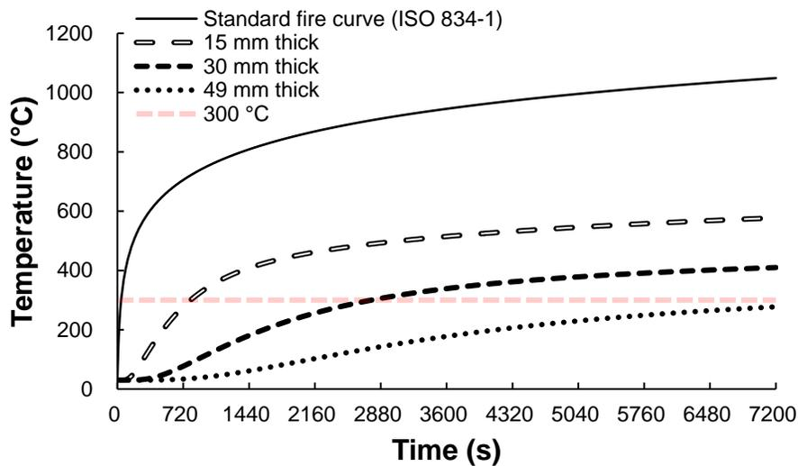
Fig. 2. Temperature-time curve of the back side of gypsum board by its thickness
