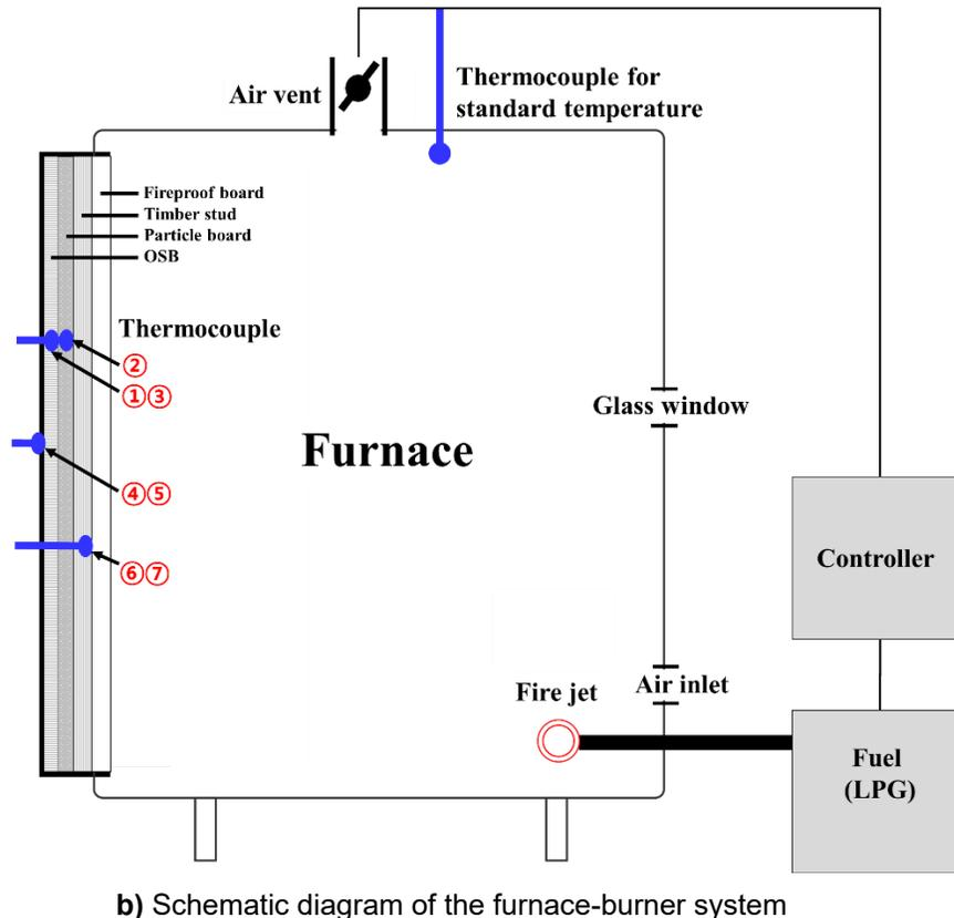
b) Schematic diagram of the furnace-burner system
