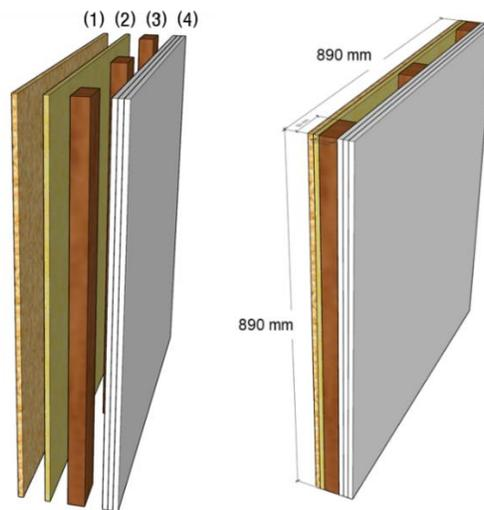
**Fig. 3.** Test specimen: (1) oriented strand board, (2) particle board, (3) stud (lumber), (4) fire-resistant boards
