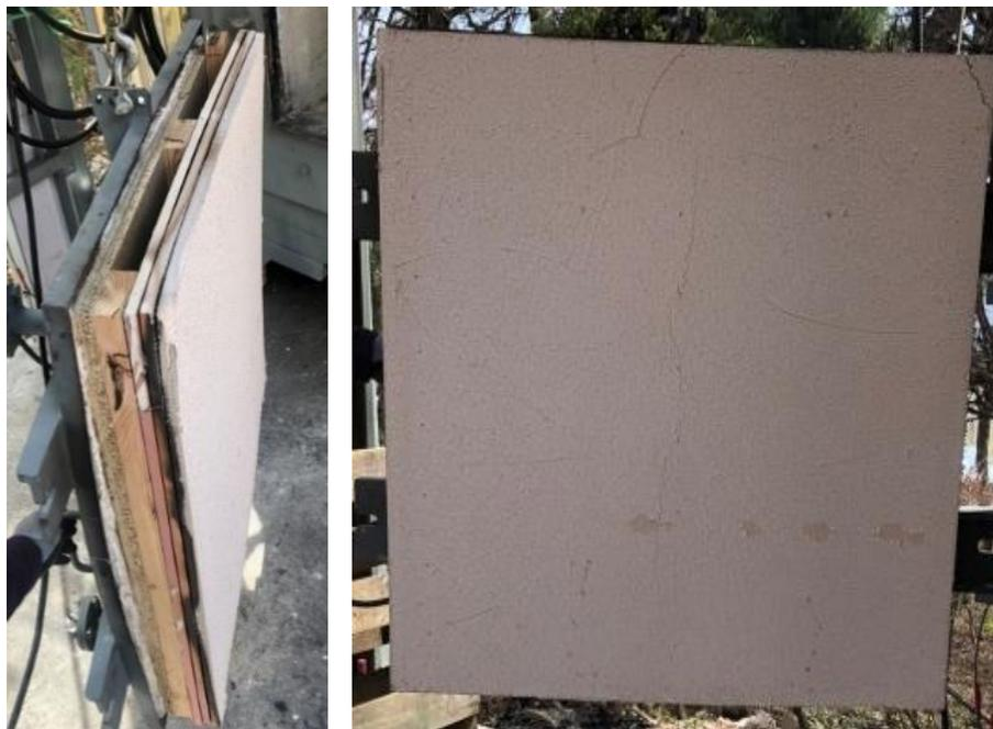
(b) Specimen after 2 h fire test
