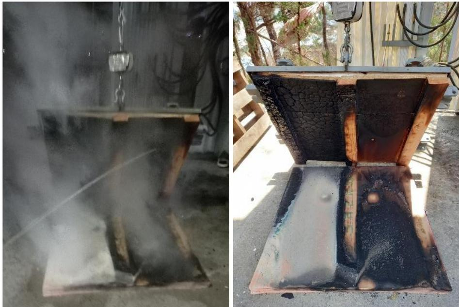
(b) Specimen after 2 h fire test
