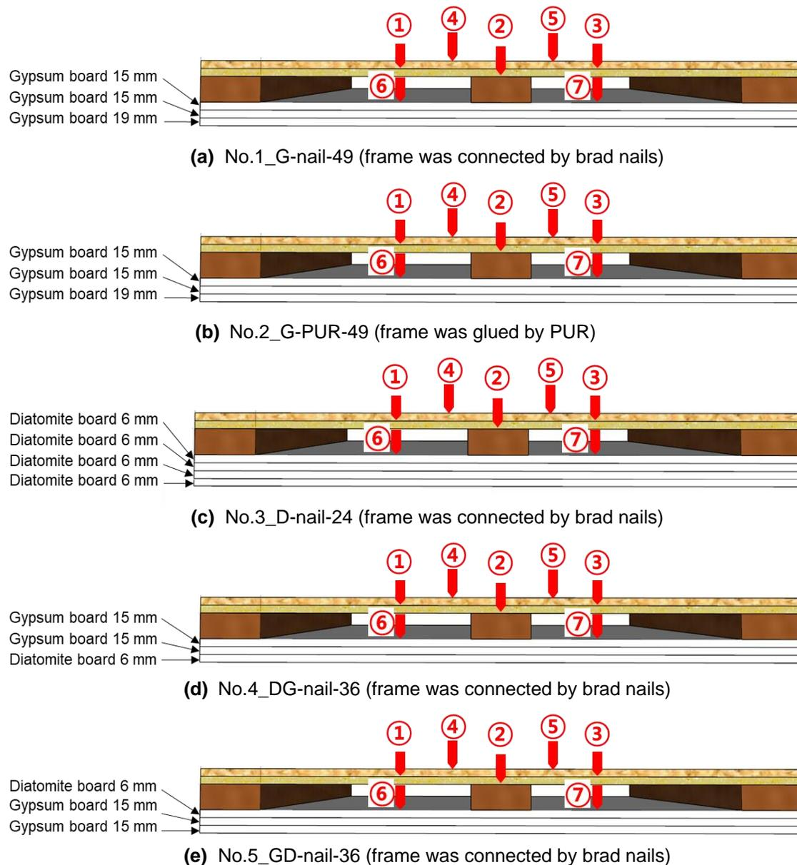
**Fig. 4.** Configuration of test specimen; the position of thermocouples, ① and ③: the back side of particle board, ②: the back of the lumber stud, ④ and ⑤: the back of OSB, ⑥ and ⑦: the back of the fire-resistant board; a: No.1 specimen, b: No.2 specimen, c: No.3 specimen, d: No.4 specimen, e: No.5 specimen
