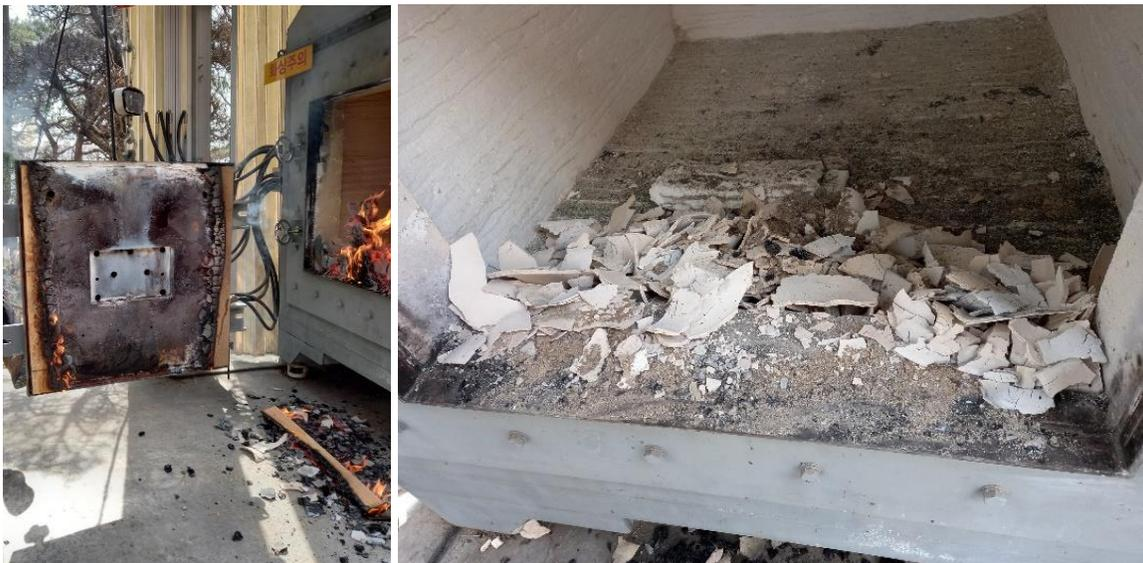
(b) Specimen after 2 h fire test
