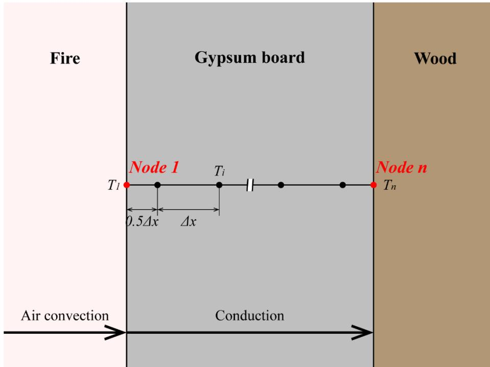
Fig. 1. The node to simulate the temperature in gypsum board by finite difference method
