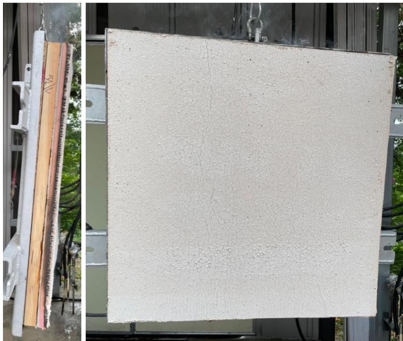
(b) Specimen after 2 h fire test
