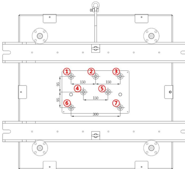
(b) Location of the thermocouples on the door of fire test chamber
