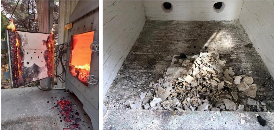
(b) Specimen after 2 h fire test
