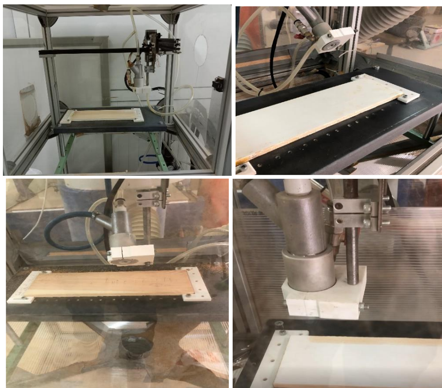
Fig. 2. Automated blasting cabinet and media blasting process
