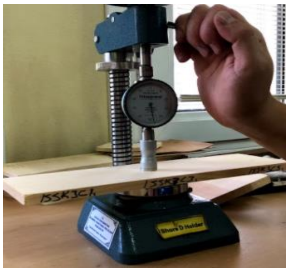
Fig. 5. Measurement of hardness values
