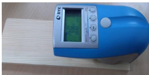
Fig. 3. Color and gloss measurement of samples
