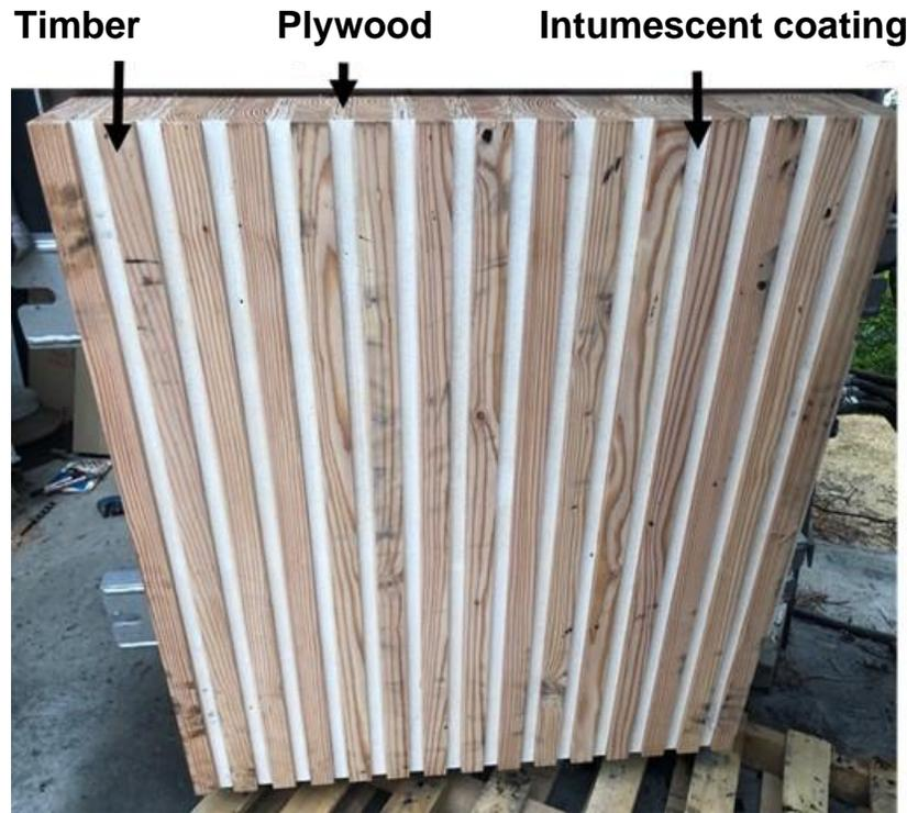
(a) Intumescent coated specimen (bottom of specimen)
