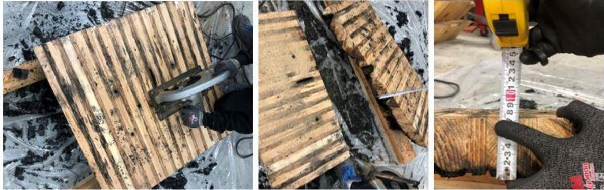
Fig. 13. Measurement of the residual depth of timber laminae
