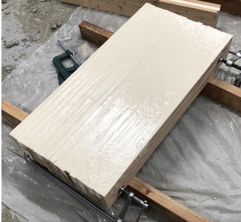
**Fig. 3.** Intumescent coating on plywood laminae
