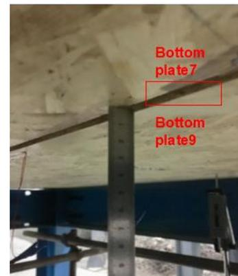
(b) Staggered layers at the bottom plate joints
