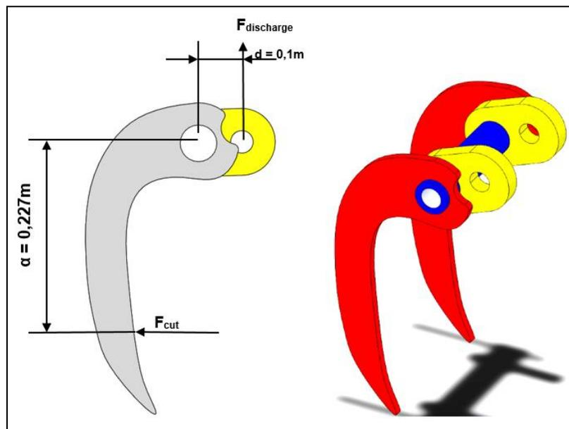
Fig. 4. Force analysis of the cutting mechanism
