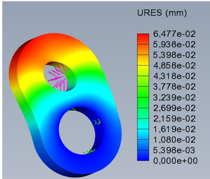
**Fig. 8.** Stress statics displacement before dimensioning the material to 15 mm
