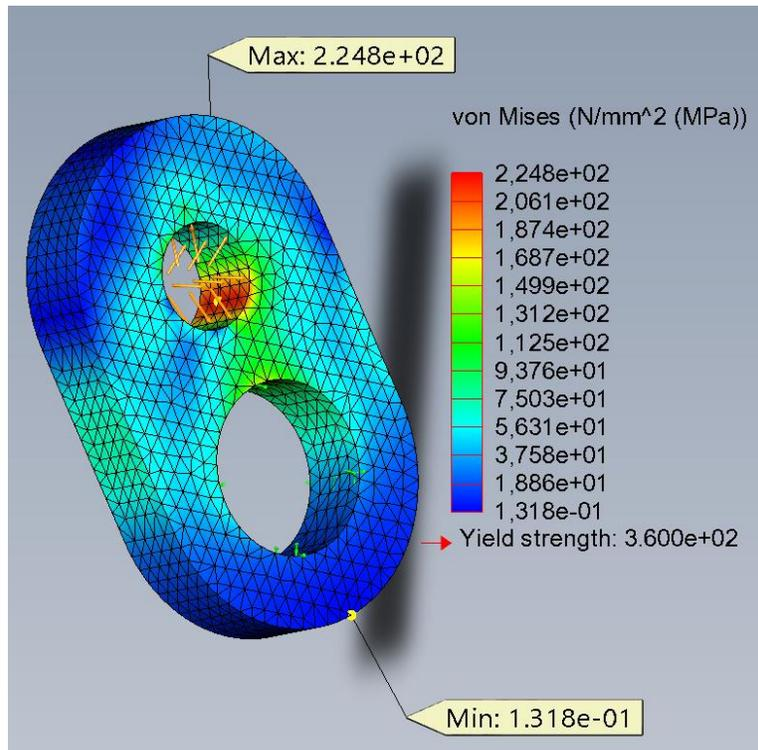
Fig. 9. The stress-strain analysis of arm the transmission
