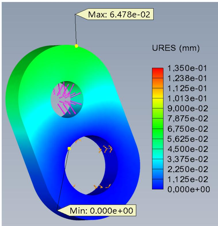
Fig. 10. The stress statics displacement after dimensioning the material to 30 mm
