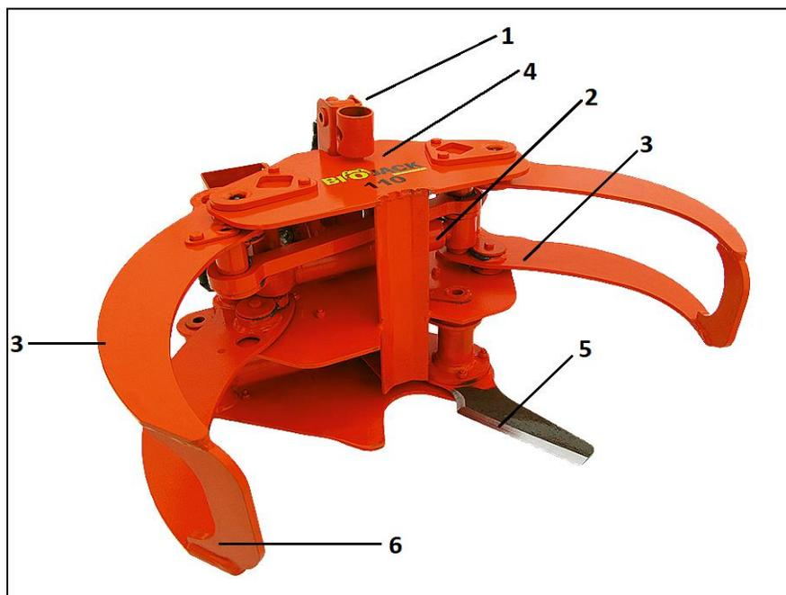
**Fig. 2.** Schematic of a chipless wood cutting head (Nisula 2022)
