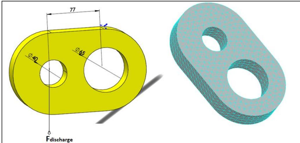
**Fig. 5.** Load diagram of the gear plate and transfer plate networking
