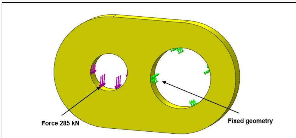
**Fig. 6.** Loading and fixed of the analyzed component of the cutting head
