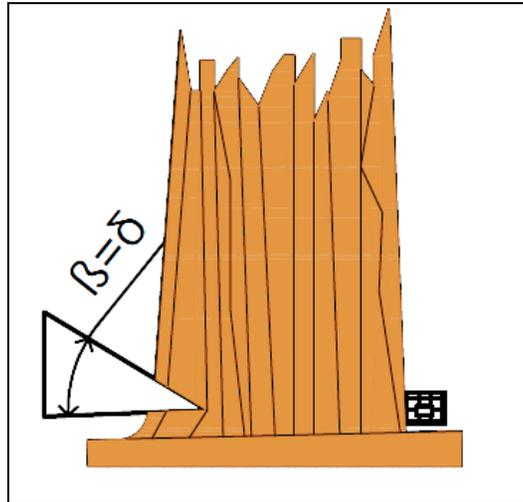
**Fig. 1.** Schematic of chipless wood cutting (Krilek *et al.* 2018)
