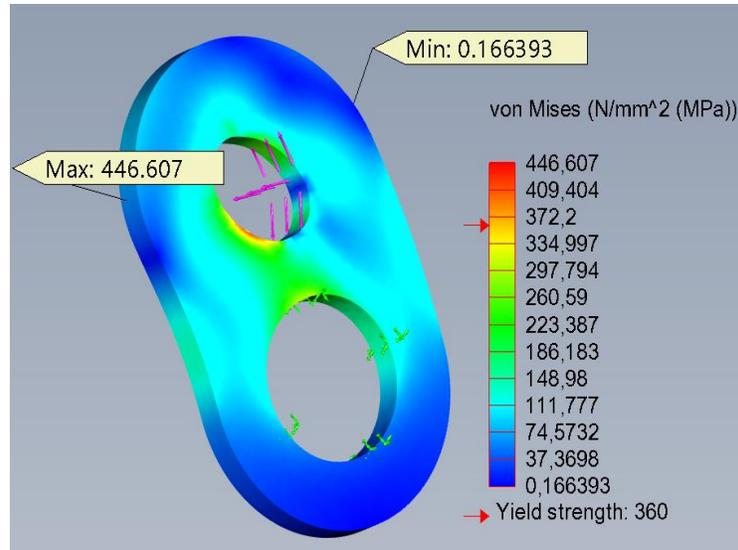
**Fig. 7.** The stress strain analysis of the arm trasmission (15 mm)
