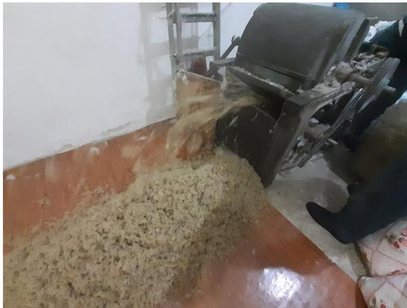
**Fig. 1.** Separation of stone wool into fibers in a wool carding machine
