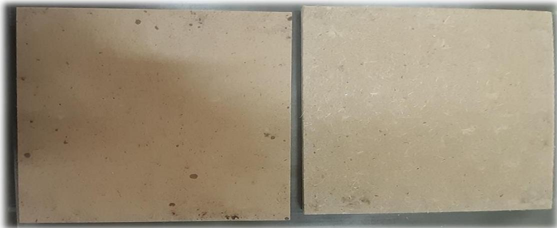
**Fig. 4.** Hybrid fiberboard samples produced from a mixture of stone wool fiber and wood fiber
