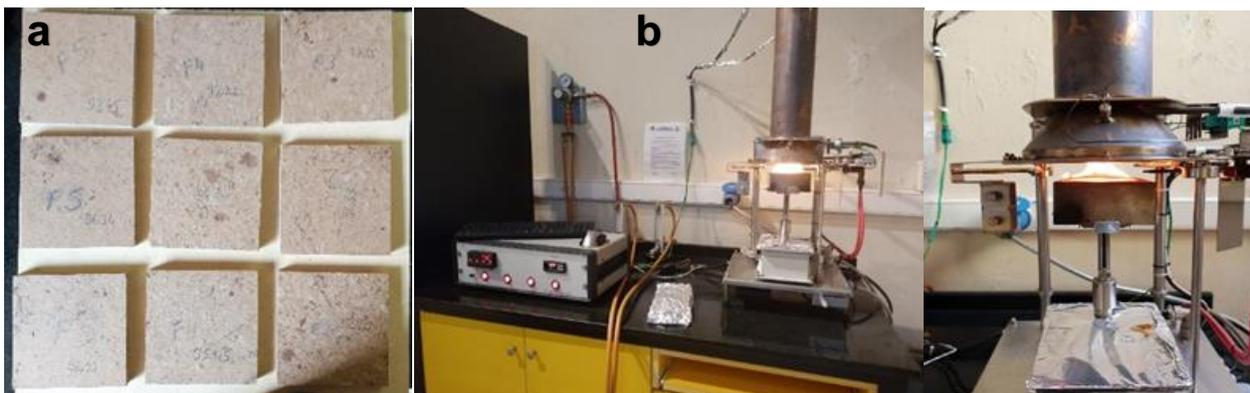
**Fig. 6.** a) Combustion test samples b) The experiment in a cone calorimeter
