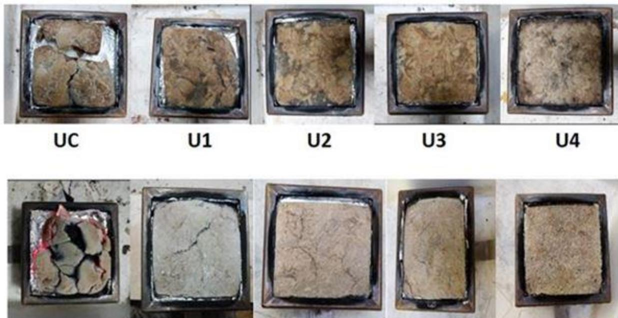
Fig. 7. Test samples after combustion
