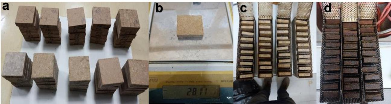
**Fig. 5.** a) Test samples b) The weighing of test samples c) The putting of test samples in the wireframe d) Test samples after water soaking
