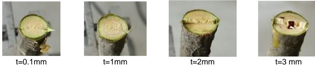
**Fig. 4.** The cutting sections with different cutting clearance
