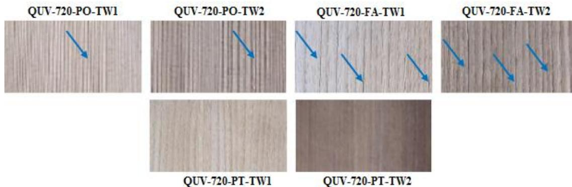
**Fig. 8.** Cracks on the surfaces of VAS samples subjected to HT after QUV
