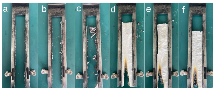
Fig. 3. The photographs of the uncoated and coated Xuan paper after vertical burning testing (a) X-0, (b) X-CS-1, (c) X-CS-5, (d) X-CS-10, (e) X-CS-15 and (f) X-CS-20
