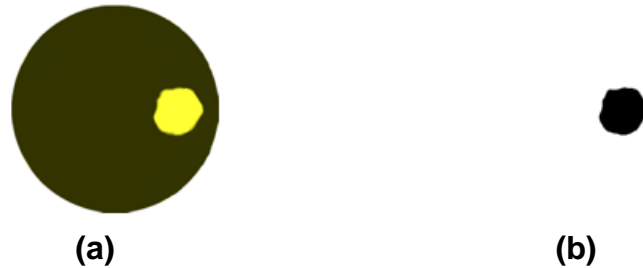
Fig. 4. Example of Roi (b) generated from tomographic image (a) of the defect
