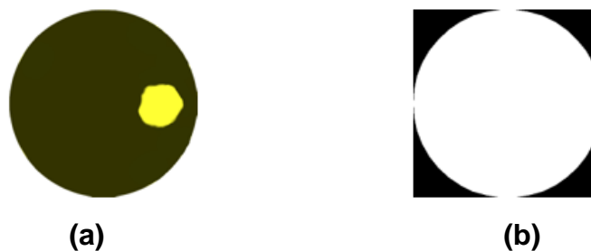
Fig. 6. Example of internal points (b) generated from the tomographic image of the simulated defect (a)
