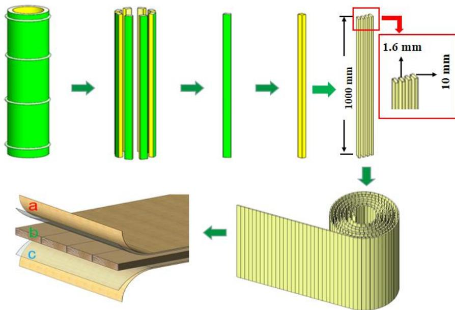
**Fig. 1.** The composition unit and structure of bamboo filament decorative board. (a) Decorative bamboo filament; (b) Chinese fir finger-joint; (c) MUF impregnated adhesive paper
