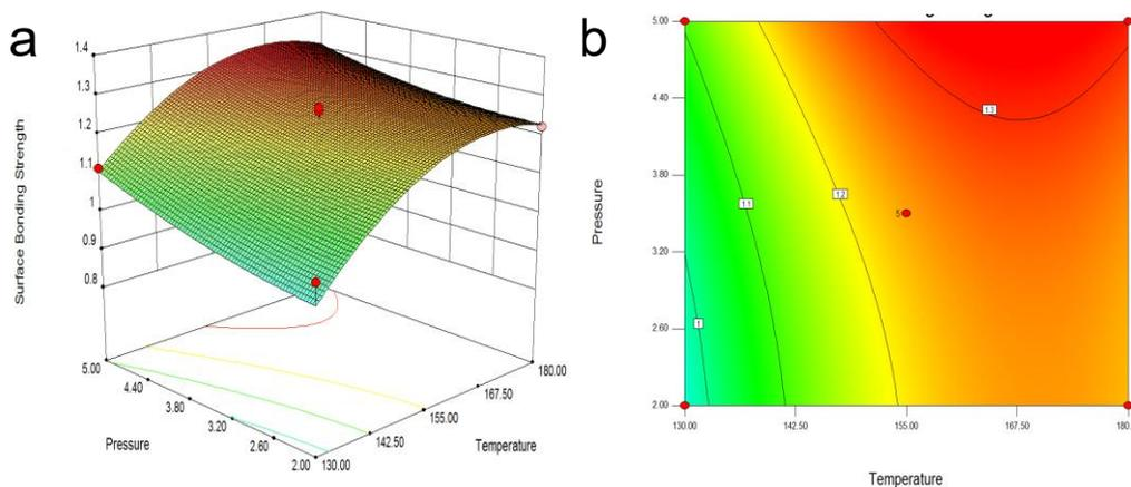
**Fig. 7.** Response surface and contour plot for hot pressing pressure and temperature on the surface bonding strength of bamboo filament decorated board
