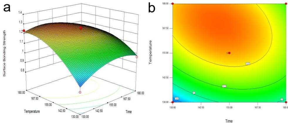
**Fig. 5.** Response surface and contour plot for hot pressing time and temperature on the surface bonding strength of bamboo filament decorated board
