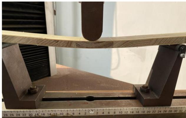
**Fig. 3.** The Static Bending Strength Test of bamboo filament decorative board
