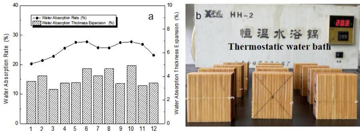
**Fig. 9.** Water absorption and thickness expansion rate test
