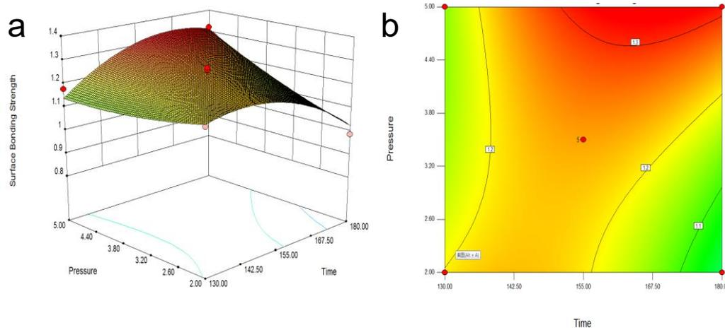
**Fig. 6.** Response surface and contour plot for hot pressing time and pressure on the surface bonding strength of bamboo filament decorated board
