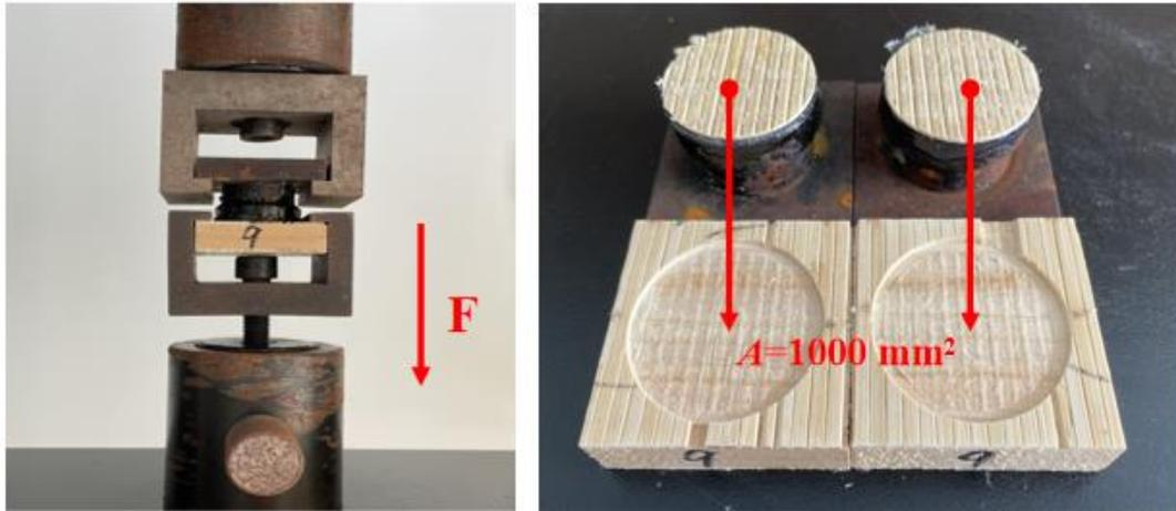
**Fig. 2.** The surface bonding strength test of bamboo filament decorative board
