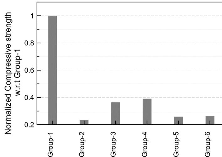
**Fig. 8.** Normalized compressive strength of the concrete of each group with respect to (w.r.t) Group-1 (NC-CTRL1)
