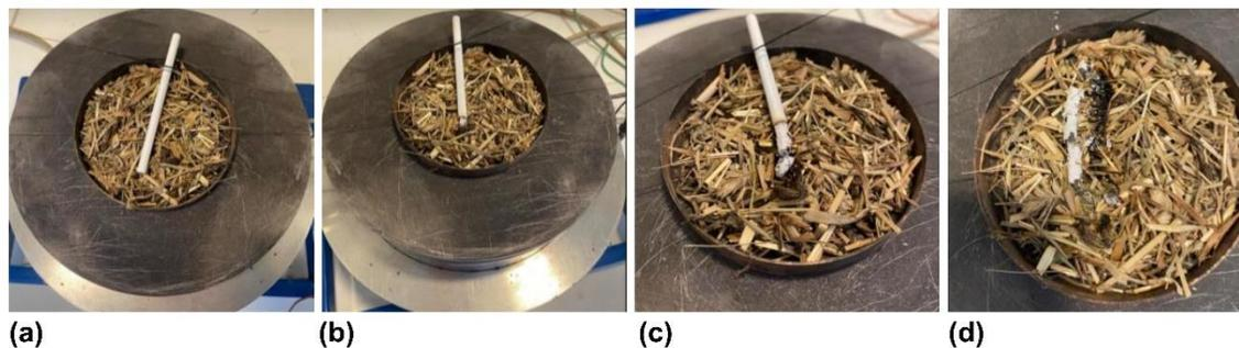
**Fig. 13.** Demonstration of the burning cigarette experiment. Key: (a) before experiment; (b) experiment at 1 min; (c) experiment at 3 min; (d) specimen at 5 min, after experiment.
