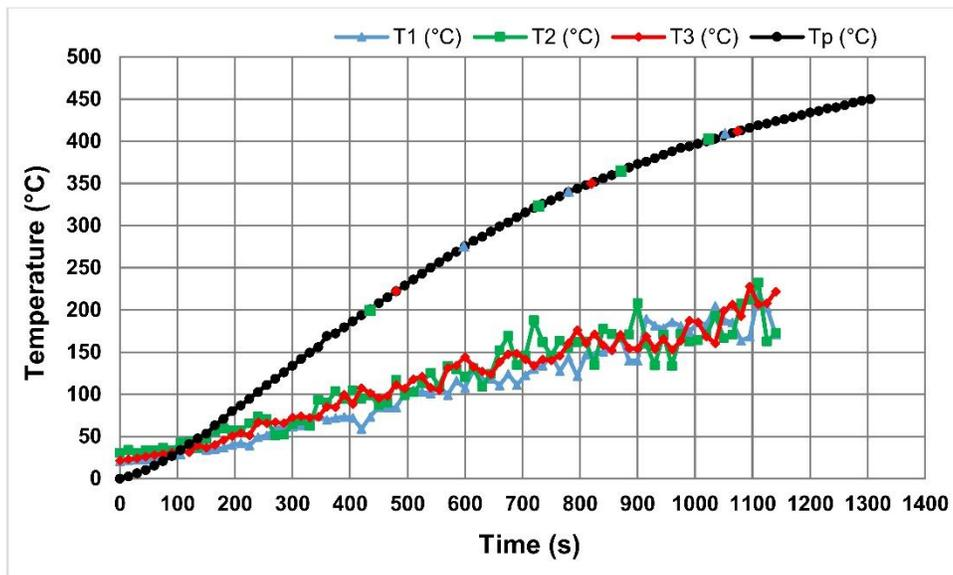
**Fig. 12.** Time-temperature curves obtained by thermocouples of a hot plate device.
