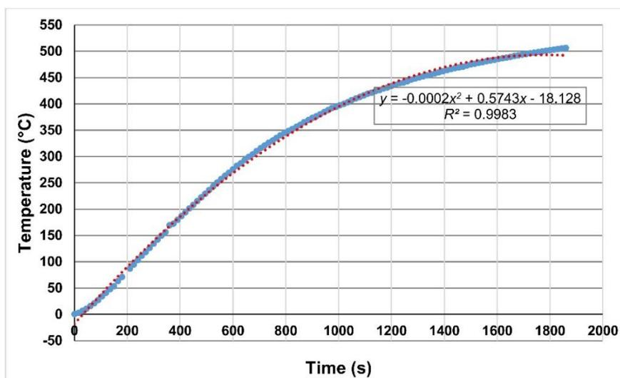
**Fig. 10.** Dependence of the temperature rise of the hot plate surface on time
