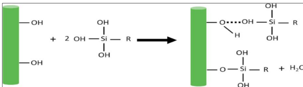
Fig. 8. Reaction of silane with NFr (R representing organic group, ... representing hydrogen bonding) (Islam et al. 2021; Creative Commons Attribution (CC BY 4.0))
