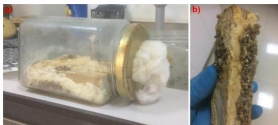
**Fig. 1.** Images for: a) heterogeneous and b) homogeneous colonization of wood samples by *P. vitreus* fungus in glass jars
