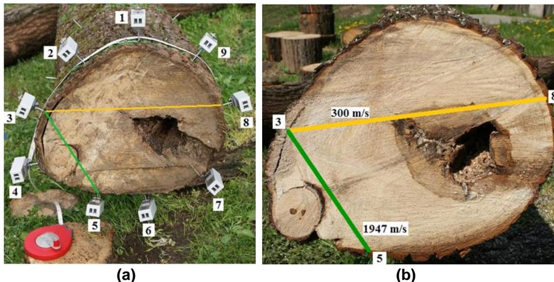
**Fig. 3.** Extreme values of the speed of sound propagation through wood: a) location of the sensors at the analyzed section; b) directions of sounds propagation
