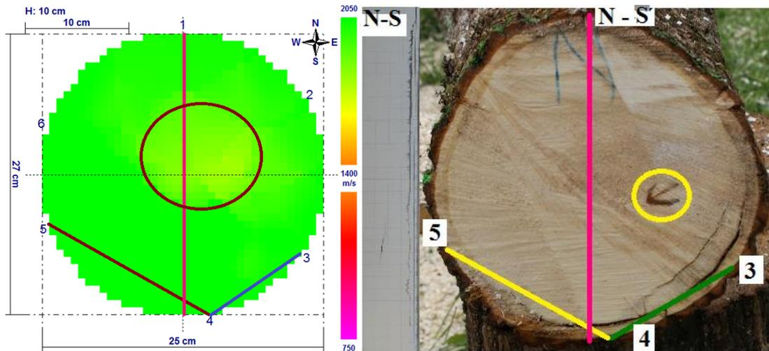
Fig. 14. Failure to recognize the knot on the 10 cm section of the third piece of wood
