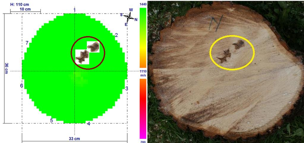
Fig. 10. Tomogram and section from 110 cm to the first piece of lime
