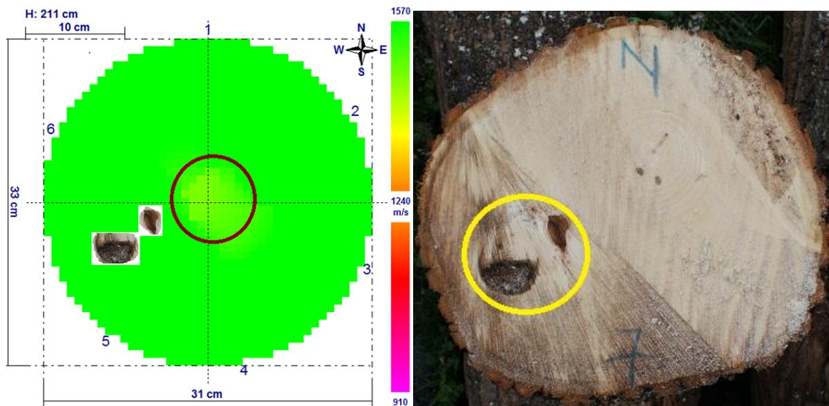
Fig. 11. Tomogram and section from 211 cm to the first piece of lime
