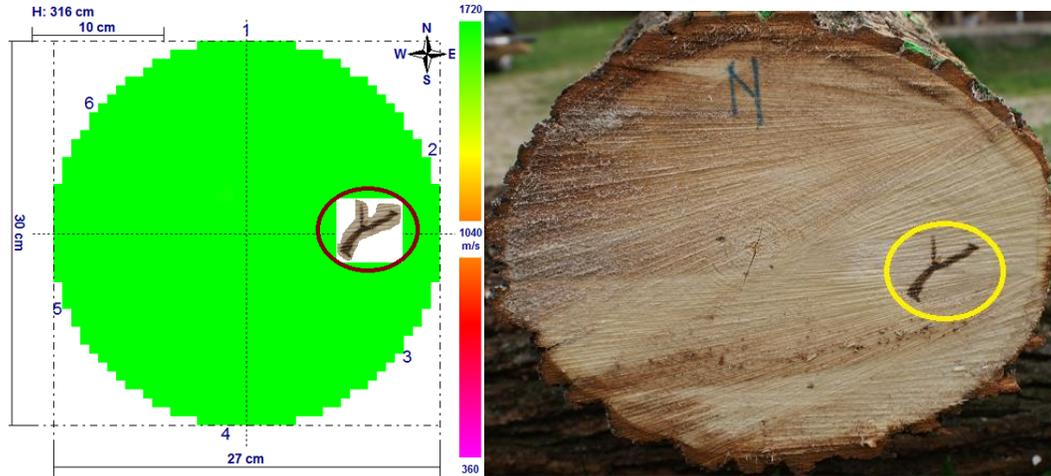
Fig. 12. Tomogram and section from 316 cm to the first piece of lime
