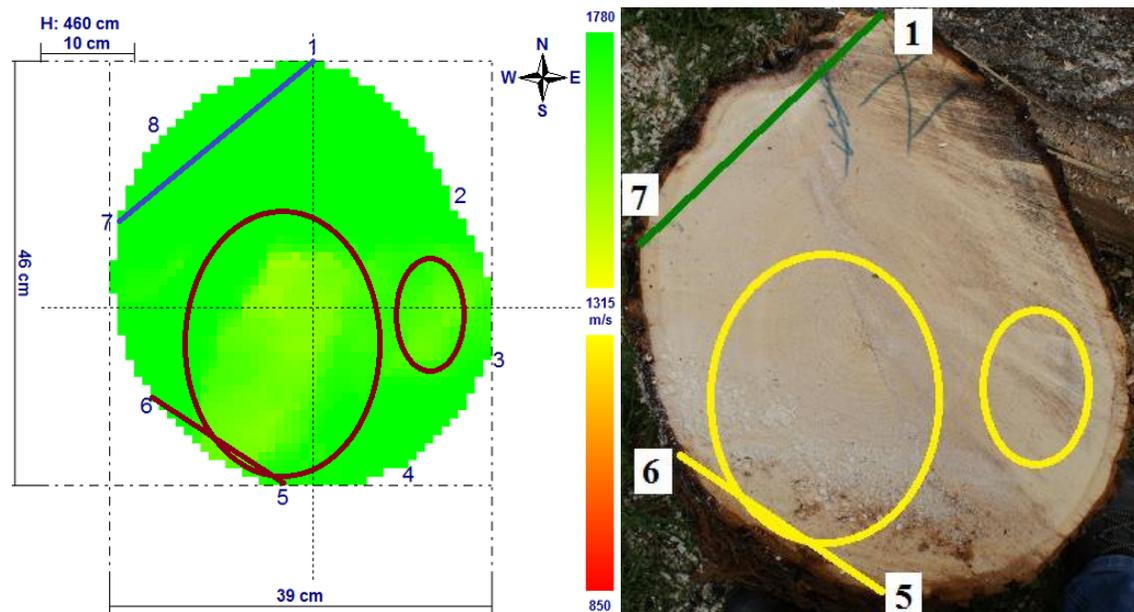
**Fig. 9.** Speeds of sound propagation through a portion with wide annual rings
