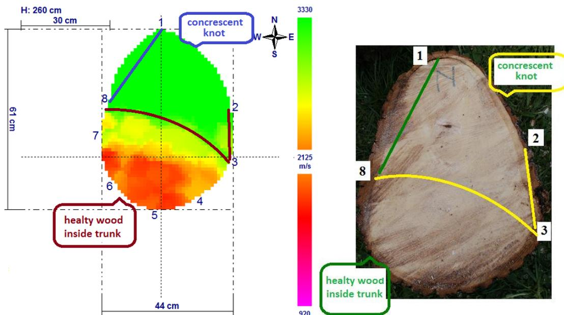
Fig. 20. Propagation of sounds through the trunk and through a healthy knot (the first piece)
