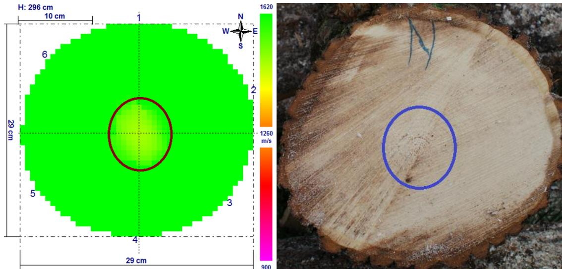
**Fig. 8.** The influence of wood density from the center of the trunk on the sound speeds
