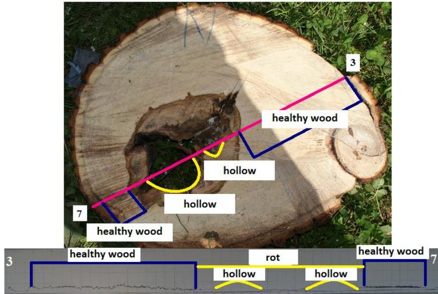
Fig. 19. The diagram of relative resistance to drilling registered between sensors 7-3
