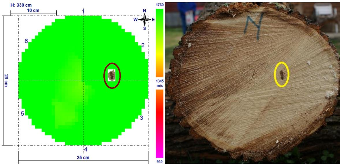
Fig. 13. Tomogram and section from 330 cm to the first piece of lime
