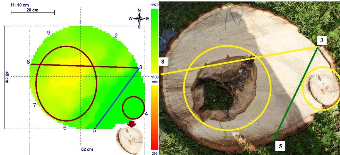
Fig. 17. Identifying a hollow and a rotten area
