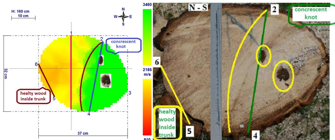
**Fig. 21.** Propagation of sounds through the trunk and through a healthy/living knot (the third piece)
