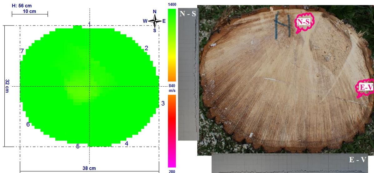
Fig. 4. The results from the level of 56 cm of the first piece of lime
