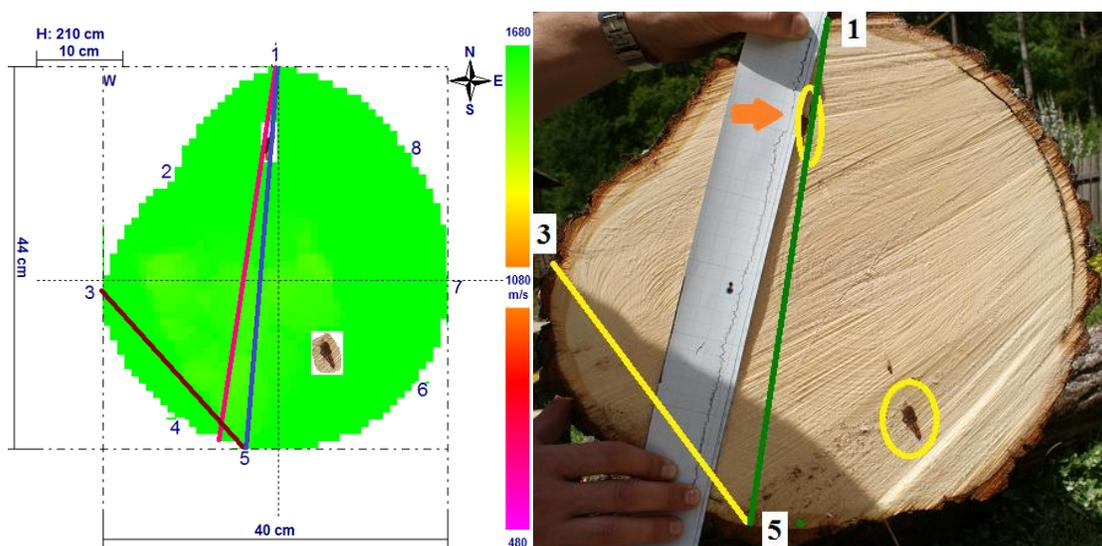
Fig. 16. Failure to identify defects on the 210 cm section at the second piece of wood
