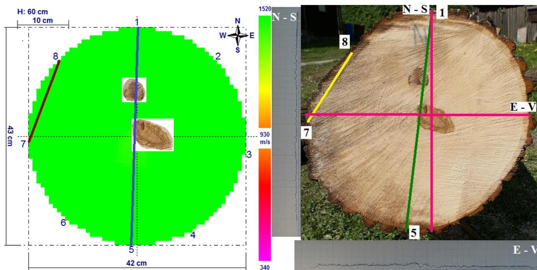
Fig. 15. Non-identification of defects on the 60 cm section at the second piece of wood
