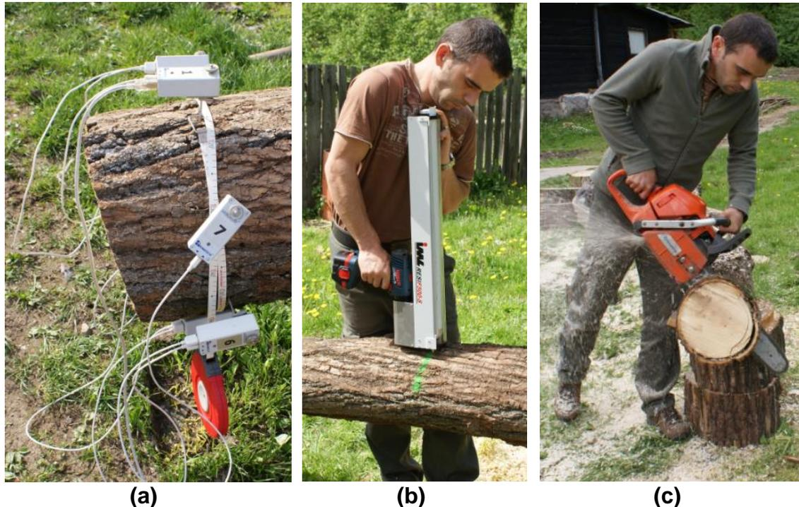
**Fig. 1.** The field sampling: a) the sensors were placed around the wood piece for acoustic analyses; b) the measurements were made by a wood drilling machine; c) the cross-cut for evaluating the true status of the wood
