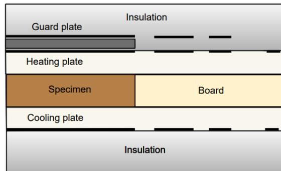
**Fig. 1.** Half-diagram of the single-specimen guarded heated plate apparatus
