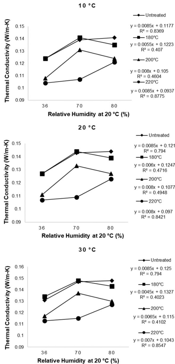
**Fig. 3.** Thermal conductivity of untreated and HTB specimens at mean plate temperatures of 10 °C, 20 °C, and 30 °C as a function of relative humidity
