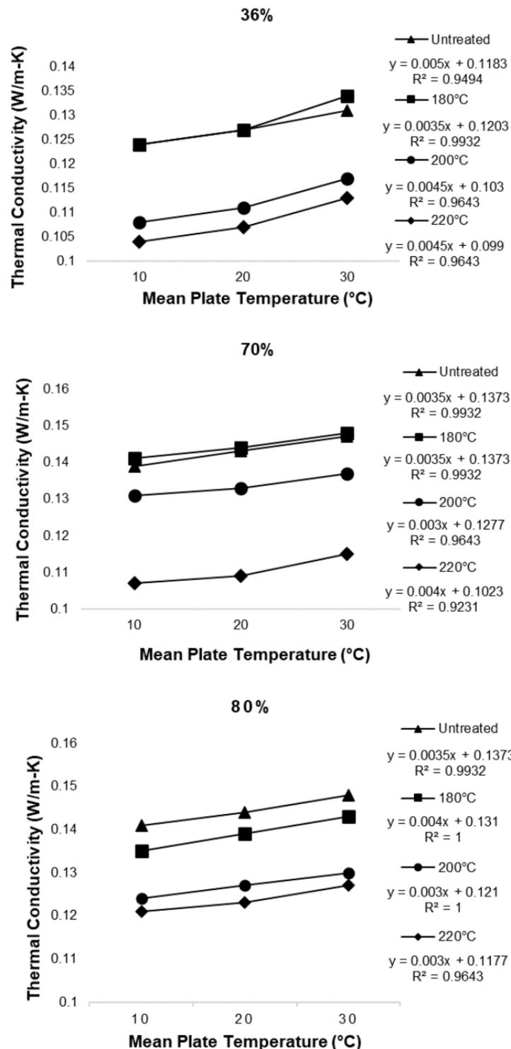
**Fig. 7.** Thermal conductivity of untreated and HTB specimens at three different moisture conditions of 36%, 70%, and 80% as a function of mean plate temperature
