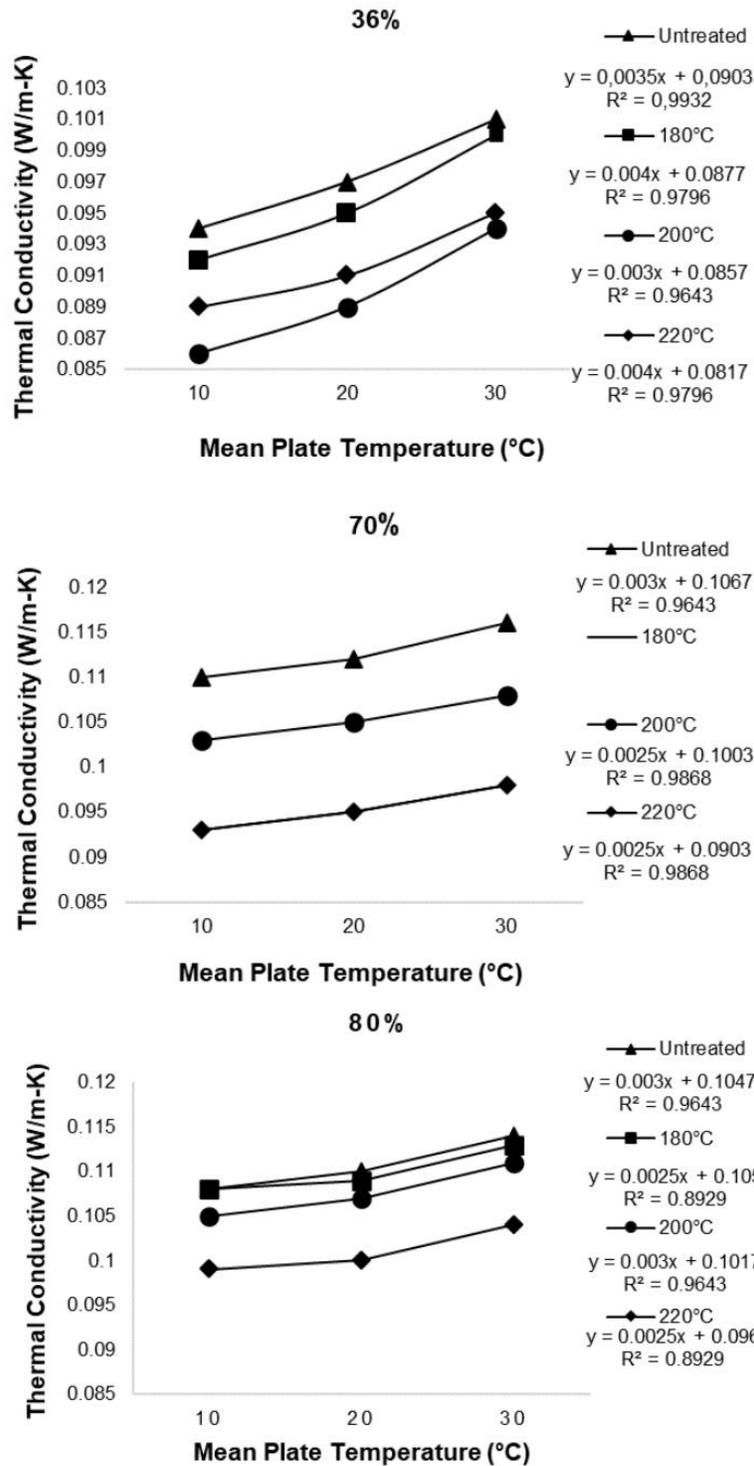
**Fig. 6.** Thermal conductivity of untreated and HTP specimens at three different moisture conditions of 36%, 70%, and 80% as a function of mean plate temperature
