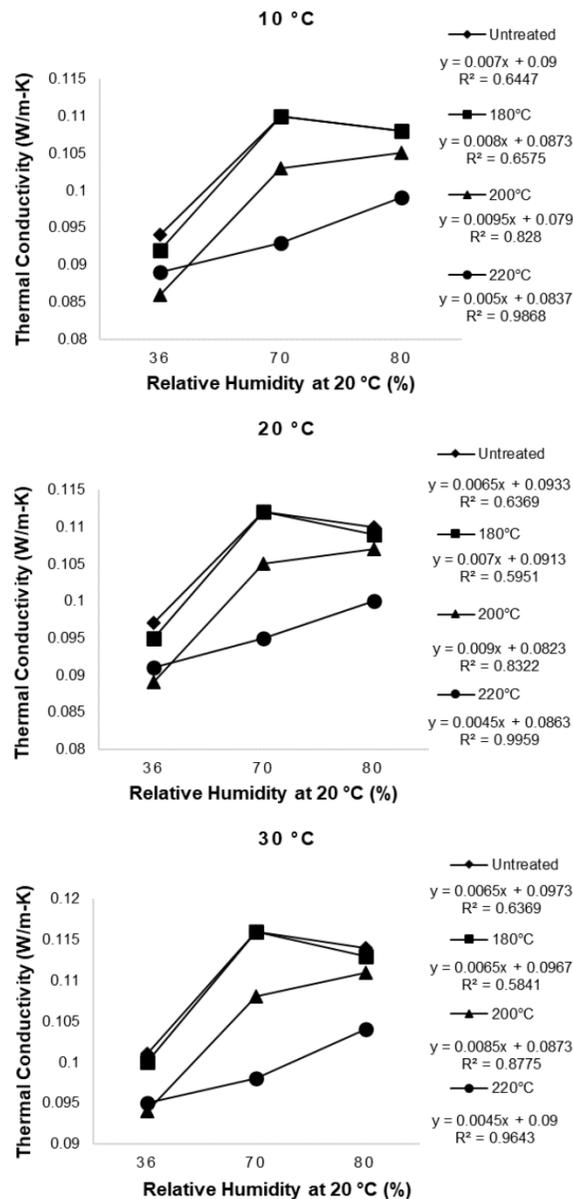
**Fig. 2.** Thermal conductivity of untreated and HTP specimens at mean plate temperatures of 10 °C, 20 °C, and 30 °C as a function of relative humidity
