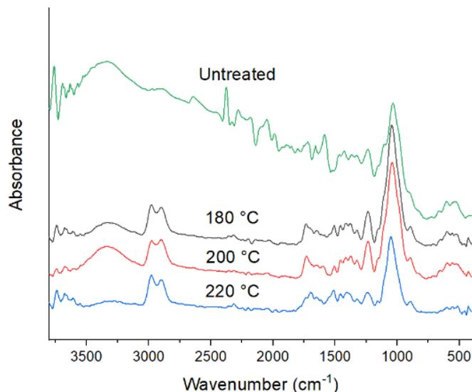
Fig. 4. FTIR spectra of untreated and heat-treated beech wood
