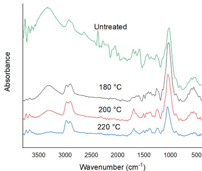
Fig. 5. FTIR spectra of untreated and heat-treated pine wood
