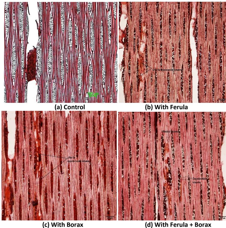
**Fig. 5.** Appearance of retention in tangential sections of impregnated mahogany wood
