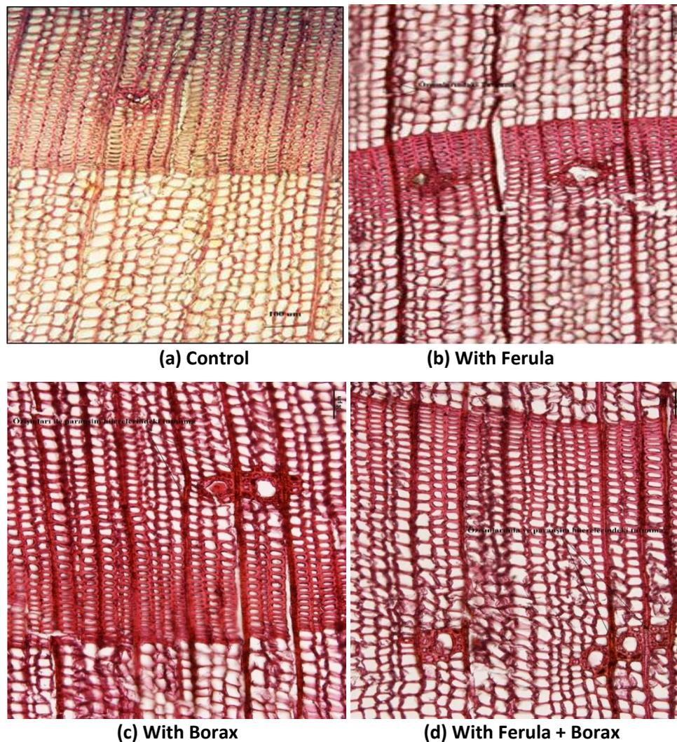
**Fig. 1.** The appearance of retention in cross-sections of impregnated eastern spruce wood
