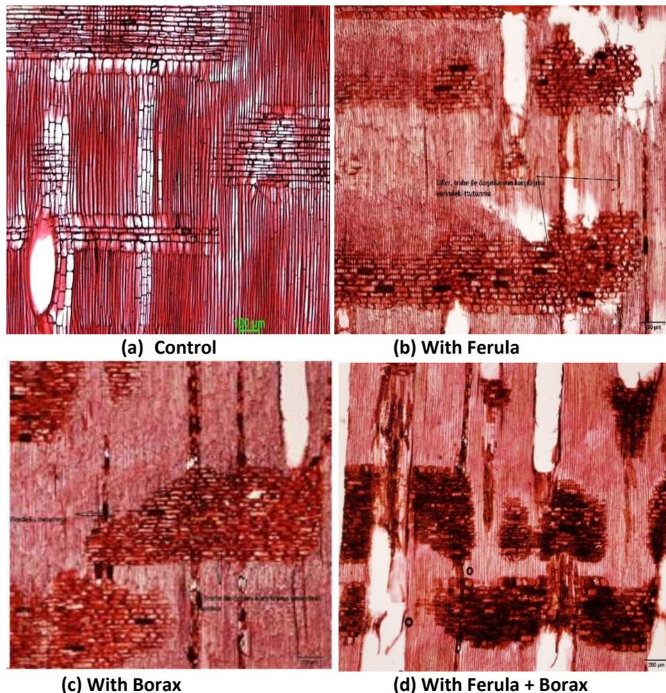
**Fig. 6.** Appearance of retention in radial sections of impregnated mahogany wood
