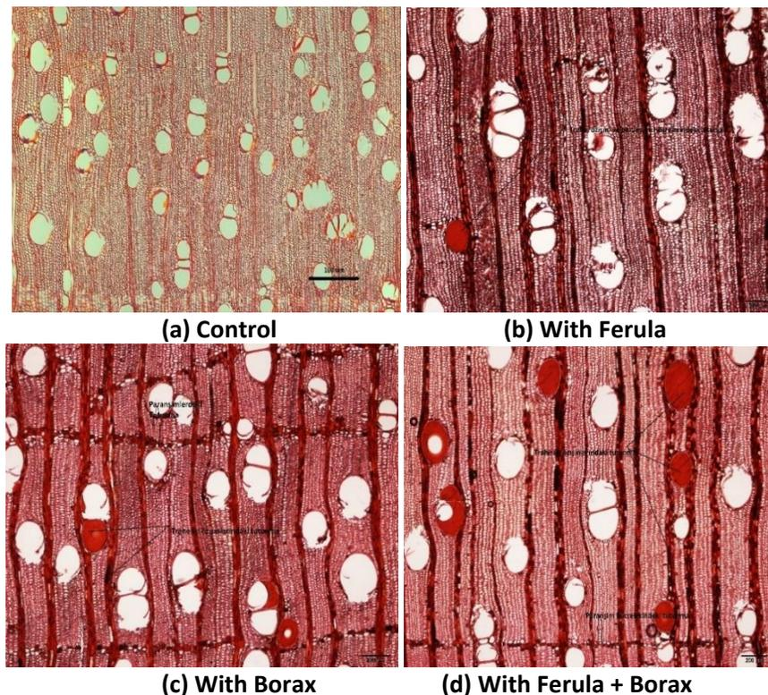
**Fig. 4.** Appearance of retention in cross-sections of impregnated mahogany wood
