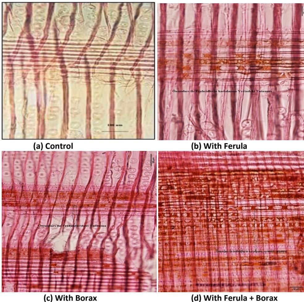
**Fig. 3.** Appearance of retention in radial section of impregnated eastern spruce wood
