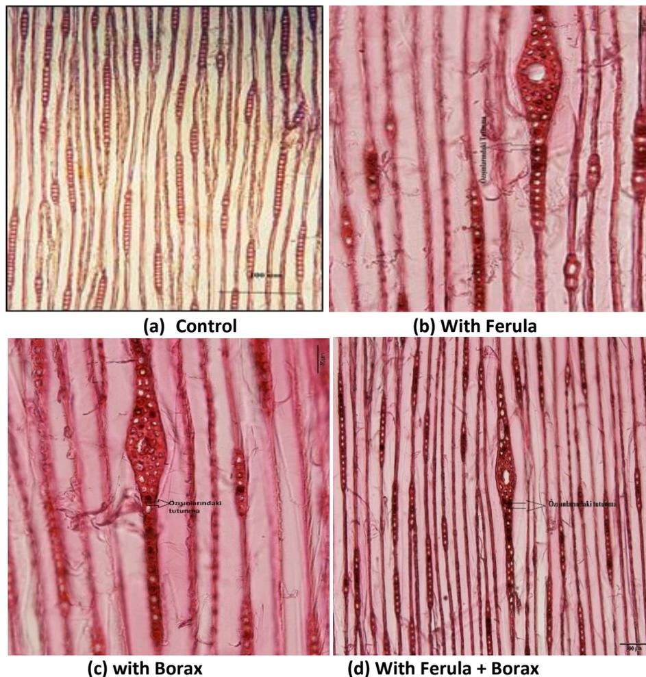
**Fig. 2.** The appearance of retention in tangential sections of impregnated eastern spruce wood
