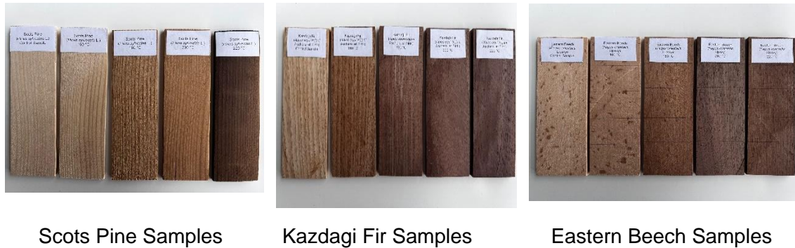
Fig. 3. Thermal modified Scots pine, Kazdagi fir, and Eastern beech species, control, 160 °C, 180 °C, 200 °C, and 220 °C respectively
