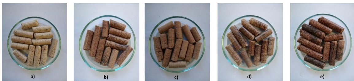
Fig. 2. The formed pellets: a) 100 Spruce pellets; b) 50 Pistachio; c) 100 Pistachio; d) 50 Peanut; and e) 100 Peanut
