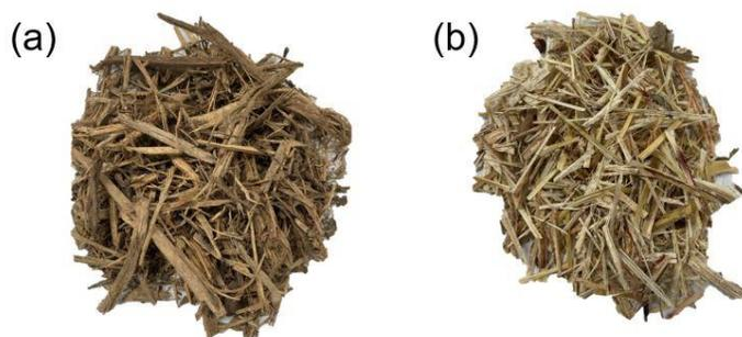
Fig. 1. Shapes of logging residue (a) and sweet sorghum samples (b) for moisture measurement
