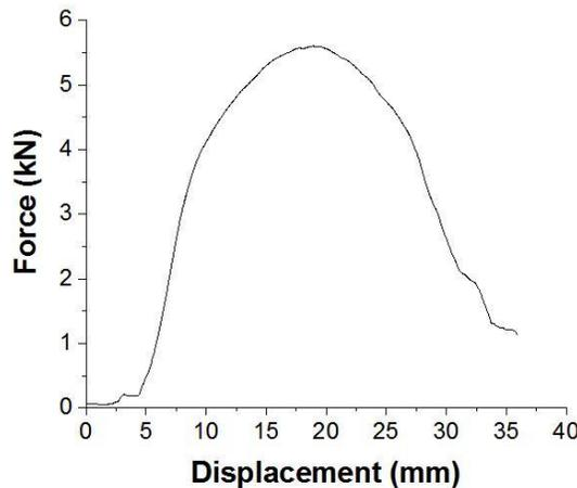
Fig. 7. Load bearing curve of the single shear joint with twist nail connection
