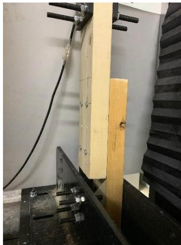
**Fig. 4.** Tensile testing setup for the single shear specimens of wooden nail welding
