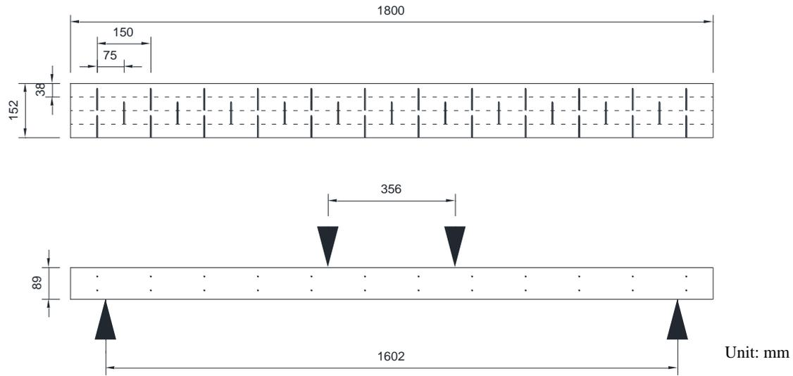
**Fig. 3.** The test method of wooden nail welding laminated timber and its bending resistance
