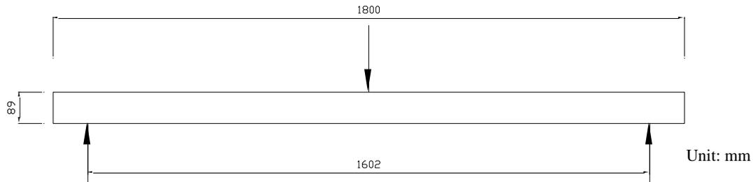
Fig. 5. Setup for the local modulus of elasticity in bending test of the laminated timber
