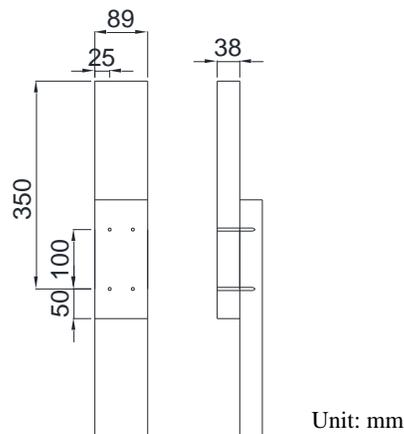
**Fig. 2.** The nailed connection single shear specimen
