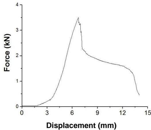
Fig. 6. Wooden nail welding single shear joint bearing curve
