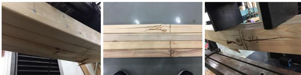
**Fig. 8.** Damage pattern of the laminated timber connected by twist nails
