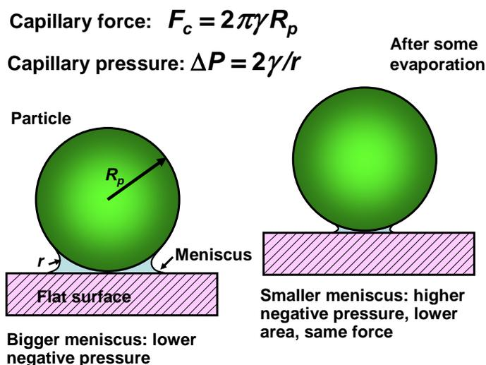
**Fig. 12.** Geometries for calculation of the capillary force based on the interfacial tension and the perimeter of water-air interfaces, which contribute to holding solid items together
