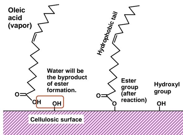
**Fig. 38.** Schematic depiction of a process of gas-phase esterification of a dry paper web to impart hydrophobicity
