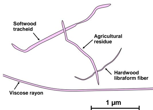
**Fig. 23.** Morphology of typical cellulosic fibers that can be considered for the preparation of filter media. The softwood, hardwood, and agricultural fiber examples are drawn from micrographs provided by Sood and Sharma (2021). Rayon fiber diameter is drawn based on the intermediate value tested by Graupner *et al.* (2018).
