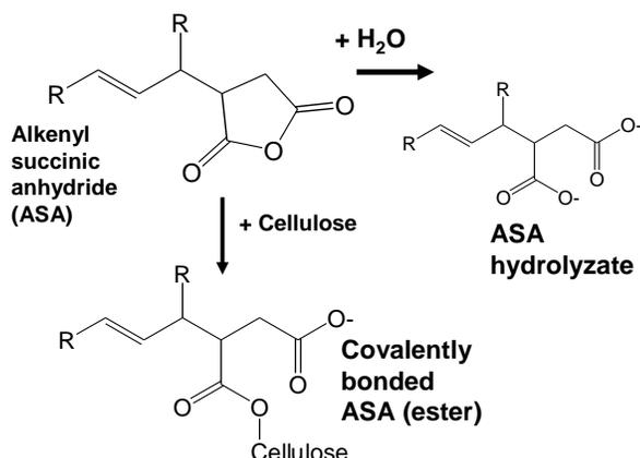
**Fig. 31.** Schematic of treatment with alkenylsuccinic anhydride (ASA) to render cellulosic surfaces hydrophobic
