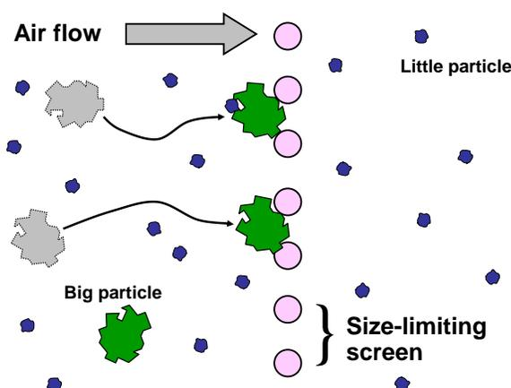
**Fig. 7.** Illustration a rudimentary screen-type capture, based on the sizes of particles relative to the size of passages between filaments in the filter medium
