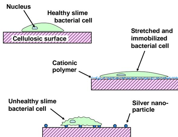
**Fig. 32.** Examples of antibacterial substances that have been shown to be effective when incorporated into cellulose-based filter media
