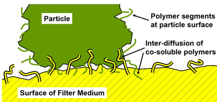
**Fig. 14.** The concept of inter-diffusion of polymer segments when the materials of two objects coming into contact have high similarity of such factors as dispersion interactions and polarity
