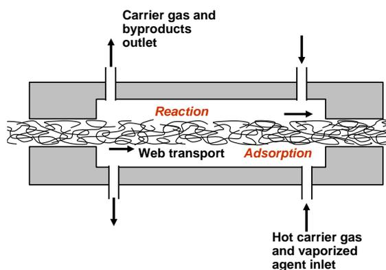
**Fig. 36.** Concept of a counter-current flow device in which hot carrier gas (to vaporize a reagent of interest) is allowed to pass over the surface of a continuously moving dry web of cellulosic material
