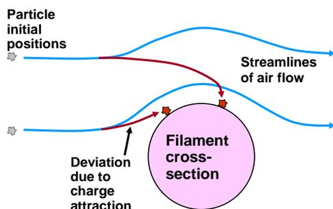
**Fig. 5.** Rudimentary illustration of an electret system that uses electrostatic attractive forces to enhance collection efficiency
