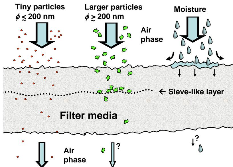
**Fig. 1.** Key attributes often wanted in media for air filtration, with a focus on facemasks. The horizontal dotted line represents a hypothetical deterministic, size-based filter structure that plays a role analogous to that of a sieve.
