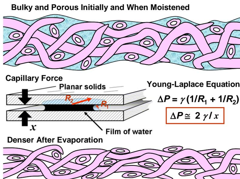
**Fig. 2.** Concept of how intermittent wetting and then drying may lead to densification and loss of void volume of cellulose-based filter media
