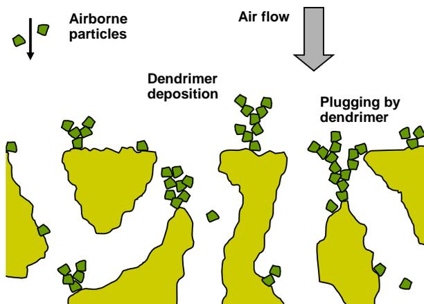
**Fig. 17.** Conceptual illustration of the formation of dendrites of collected particles within fiber-based filter media
