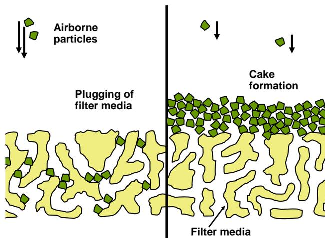
**Fig. 15.** Two ways in which the accumulation of particles can be effected to increase the pressure drop as particle-laden air passes through a porous filter
