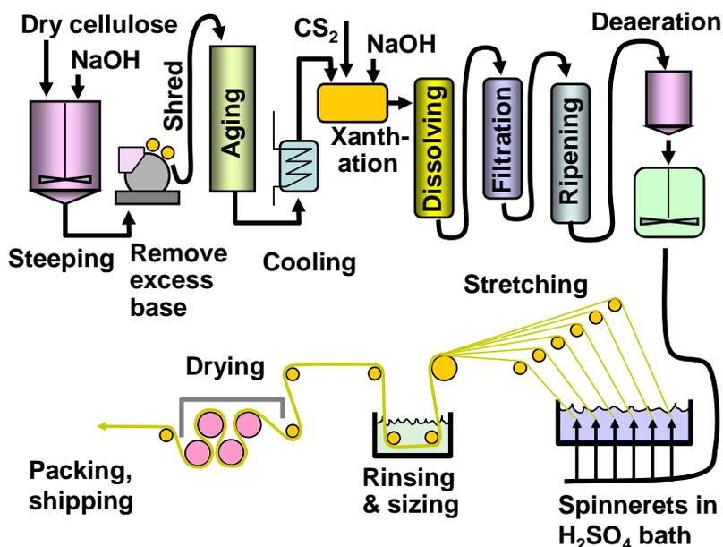
**Fig. 28.** The regeneration of cellulose to obtain fibers (viscose rayon process)
