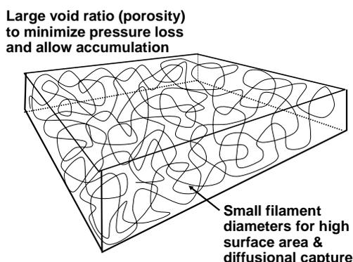
**Fig. 6.** Concept of a layer within a filter device that is designed to have a high efficiency of collection of particles by a stochastic Brownian diffusion mechanism while minimizing the resistance to air flow through the layer
