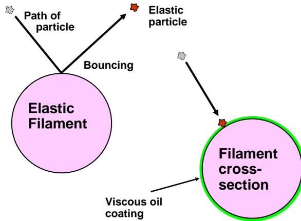
**Fig. 9.** Illustration of a viscous layer in determining whether an impinging particle will bounce from a collector surface or come to rest upon it
