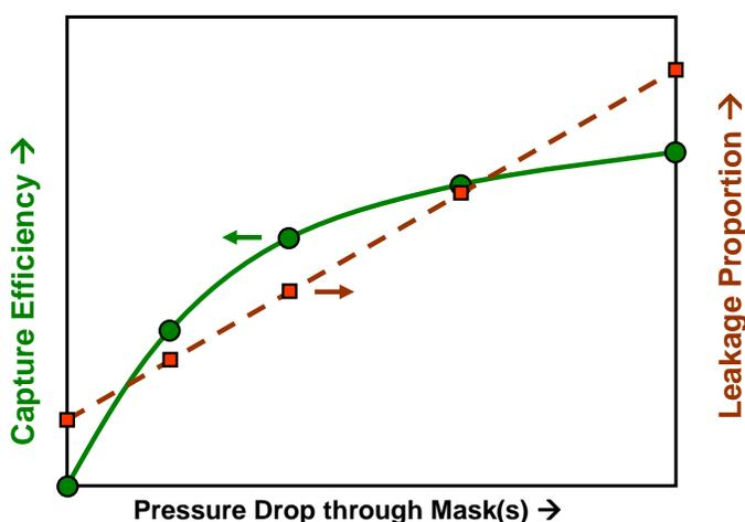
**Fig. 19.** Hypothetical illustration of an expected trade-off between collection efficiency and pressure drop, especially when using a simple uniform layer of filter media
