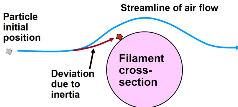
**Fig. 4.** Depiction of a deviation of particle motion from a streamline of flue due to the inertia of that particle, thus leading to a collision with a collector surface
