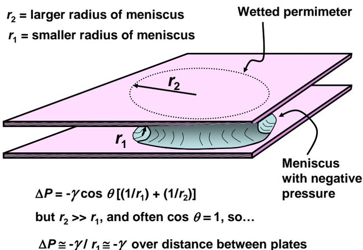
**Fig. 13.** Simplified view of a meniscus formed between a pair of flat surfaces what are envisioned as perfectly flat, featureless, and parallel, giving rise to a very strong negative pressure at the limit of close approach of the surfaces, based on the Young-Laplace equation
