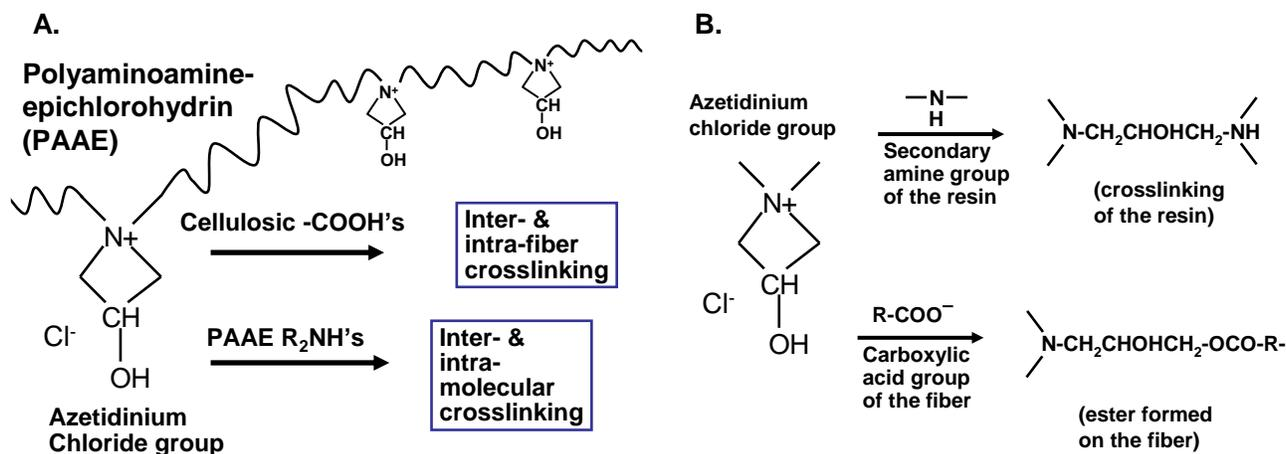
**Fig. 30.** Chemistry of the polyamidoamine-epichlorohydrin wet-strength resin system
