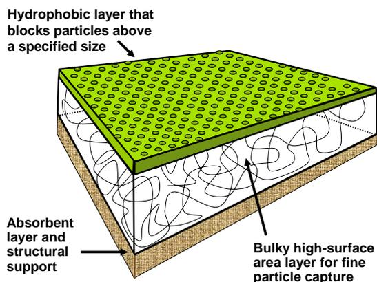
**Fig. 22.** Concept of a layered structure within a cellulose-based filter system in which one layer is specialized to resist liquid water, another is optimized to collect very small particles, and a third is designed to block large particles, absorb moisture, and provide strength to the structure
