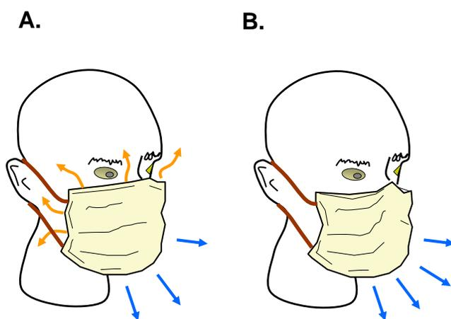
**Fig. 18.** The importance of achieving an excellent seal to prevent unfiltered air from bypassing the filter medium of a facemask. Figure concept redrawn based on original by Chiera *et al.* (2022)
