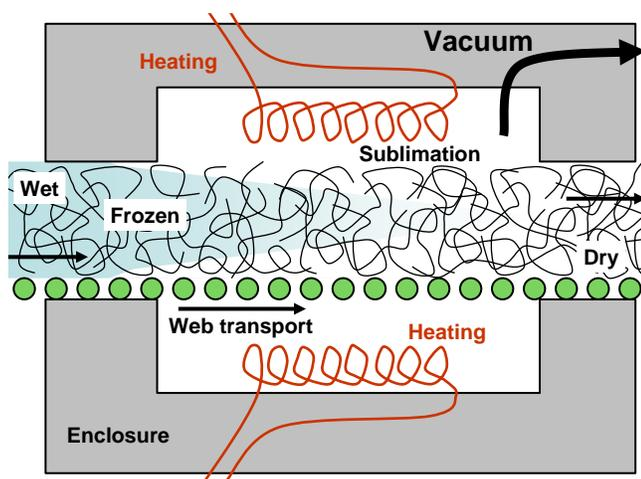
**Fig. 35.** Schematic of the freeze-drying process, which offers a way to avoid massive loss of specific surface area during the drying of nanofibrillated cellulose and related materials.
