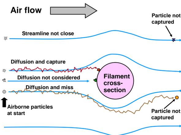
**Fig. 3.** General concept of a collection mechanism of very small particles that depends on their random (Brownian) movements due to their thermal energy, which is expressed by random collisions against gas molecules
