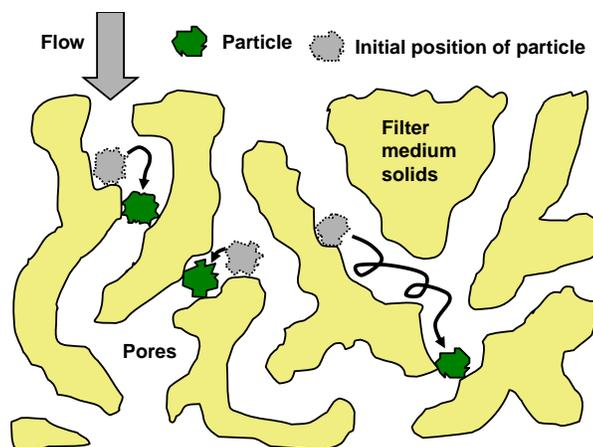
**Fig. 16.** Illustration of blockage of flow channels within porous media due to motions of unattached particles, which then become lodged at points of narrowing, which can result in a disproportionately adverse effect on flow through the material
