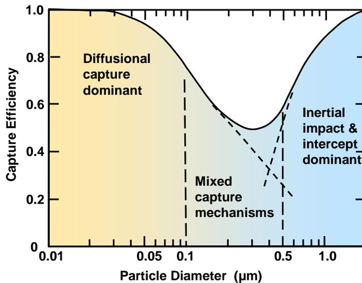
**Fig. 8.** Typical size-dependency of particle collection efficiency on filter media due to a transition from primarily stochastic (Brownian diffusion) capture to deterministic (direct impingement, momentum effects, *etc.*) at greater particle size. Figure redrawn based on original by Liu and Lee (1976)
