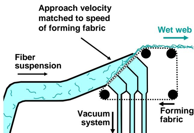
**Fig. 33.** The paper forming process, in which a suspension is dewatered on a continuous screen (in this case an inclined Fourdrinier forming device), pressed, and then dried by evaporation. Figure redrawn from US Patent 4,200,488 by Grandon *et al.* (1980)
