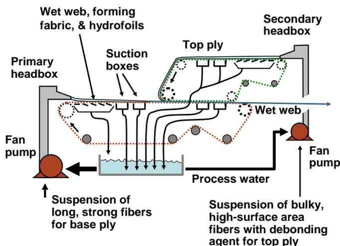
**Fig. 34.** Simplified schematic diagram of a multi-ply paper forming process, making it possible to employ specialized processing for different layers, e.g. for water repellency, stochastic collection of very small particles, and deterministic collection of intermediate-sized particles
