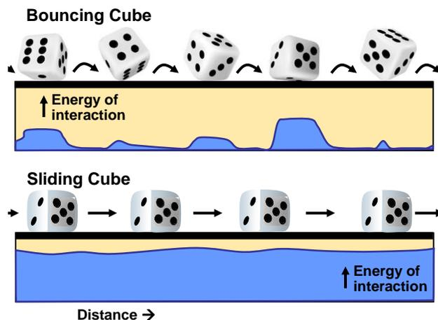
**Fig. 10.** Illustration of the contrasting ways in which a cubic particle would be expected to interact with a collector surface during an initial collision brought about by flow of particle-laden air through the device
