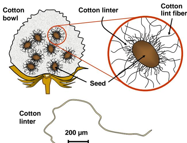
**Fig. 24.** Illustration of cotton lint (fibers) and linters present in a bowl of cotton. The illustration of the cotton bowl and its contents are redrawn based on an original from the Dieu Donn e hand papermaking company (<https://aboutabeautifulbook.wordpress.com/2015/02/28/papermaking/>). The dimensions of the individual cotton linter are based on an SEM micrograph from Luo *et al.* (2013).
