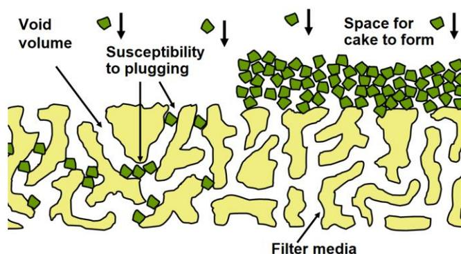
**Fig. 20.** Depiction of factors affecting the capacity of a filter device, including void volume, plugging (which can render some volume unavailable), and cake formation
