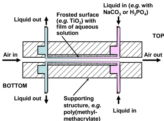
**Fig. 21.** The denuding process, which is designed to remove acid gases and ammonium from air as a means to be able to then collect semi-soluble particulates from air. Figure redrawn based on an original by Tsai *et al.* (2008)
