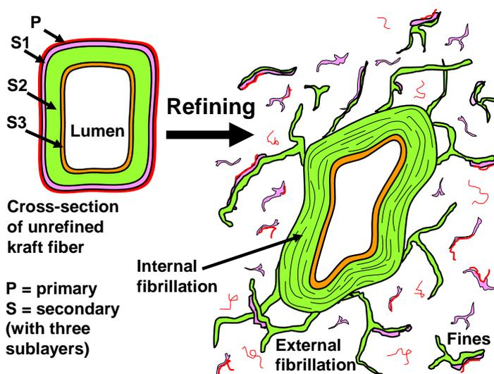
**Fig. 25.** Action of a mechanical refiner that can be used in a papermaking operation to fibrillate kraft or cotton cellulose fibers, or if used with many multiple passes can be used to prepared microfibrillated cellulose (less fibrillated than NFC). Figure adapted from Debnath *et al.* (2022)
