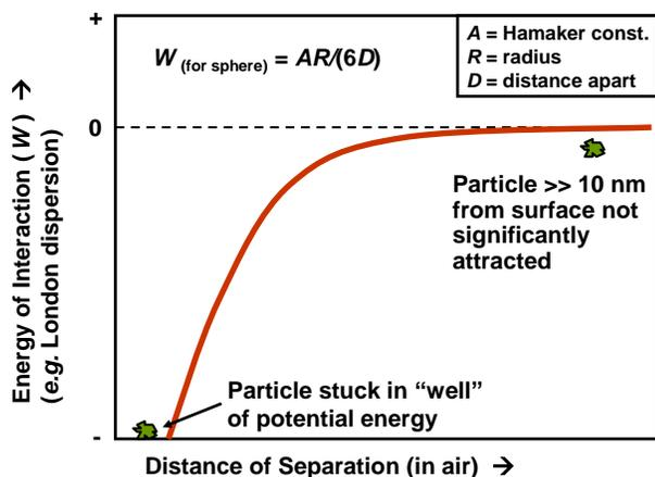
**Fig. 11.** Van der Waals (London dispersion component) energy as a function of distance between two solid objects
