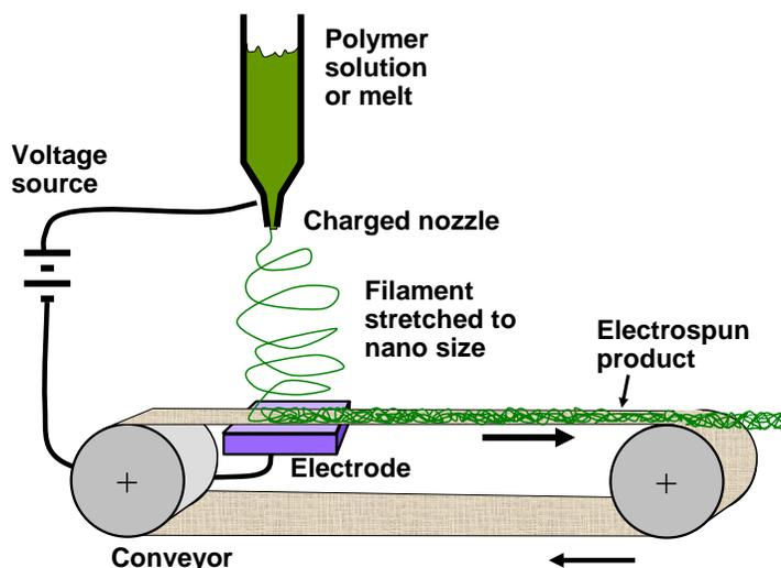
**Fig. 29.** Schematic of an electrospinning process to prepare very narrow filaments of cellulose or other polymer capable of being placed into solution and then greatly stretched during drawing
