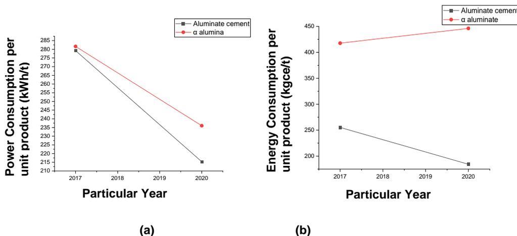
**Fig. 8.** Annual comprehensive energy consumption and power consumption change of unit product during audit period and base period: (a) Comprehensive energy consumption per unit product (b) Power consumption per unit product
