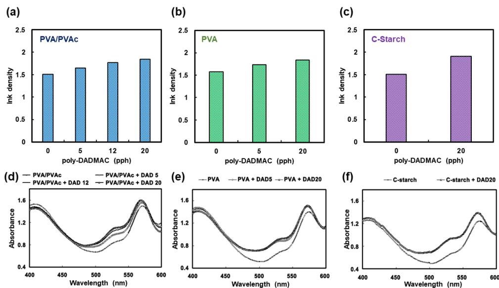
**Fig. 5.** The ink density results of the binder films where pigment-based ink was printed. Results from the densitometer of binder films consisted of (a) PVOH/PVAc, (b) PVOH, and (c) C-starch. Results from UV-Vis spectroscopy of binder films consisted of (a) PVOH/PVAc, (b) PVOH, and (c) C-starch. The ink density increased with the addition of cationic additives, regardless of the binder system.
