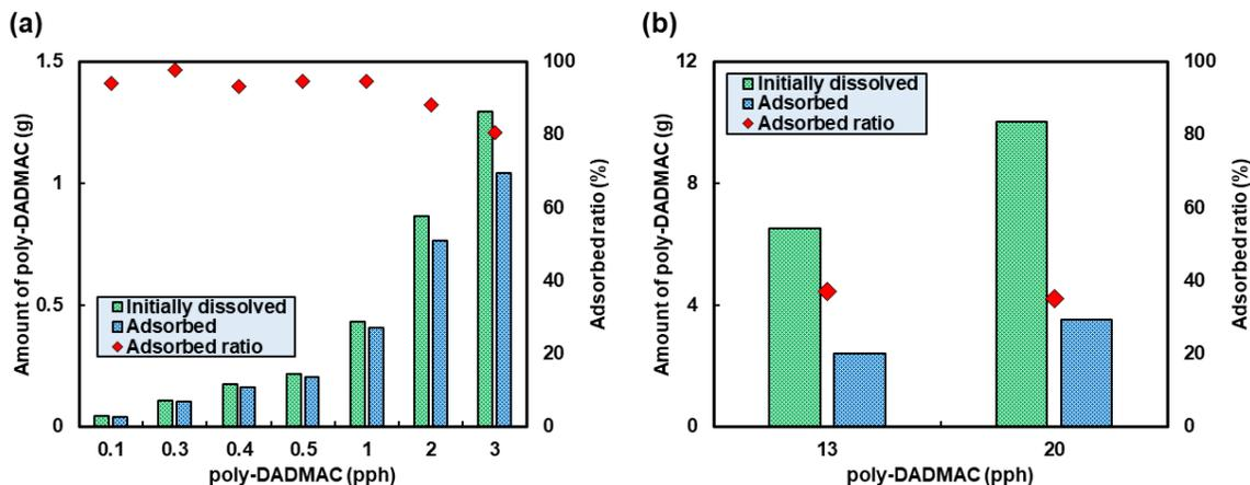
**Fig. 4.** The adsorbed amount of poly-DADMAC to silica pigments at (a) low dosage and (b) high dosage of poly-DADMAC. Adsorbed ratio = Adsorbed/Initially dissolved. (Note: the measuring methods for low and high dosages were different.)
