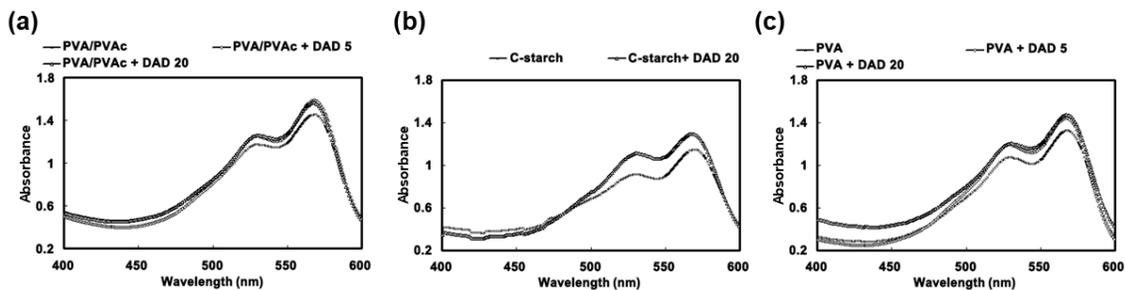
**Fig. 7.** The ink density results of the binder films where dye-based ink was printed. The UV-Vis spectroscopy of binder films consisting of (a) PVA/PVAc, (b) PVOH, and (c) C-starch.
