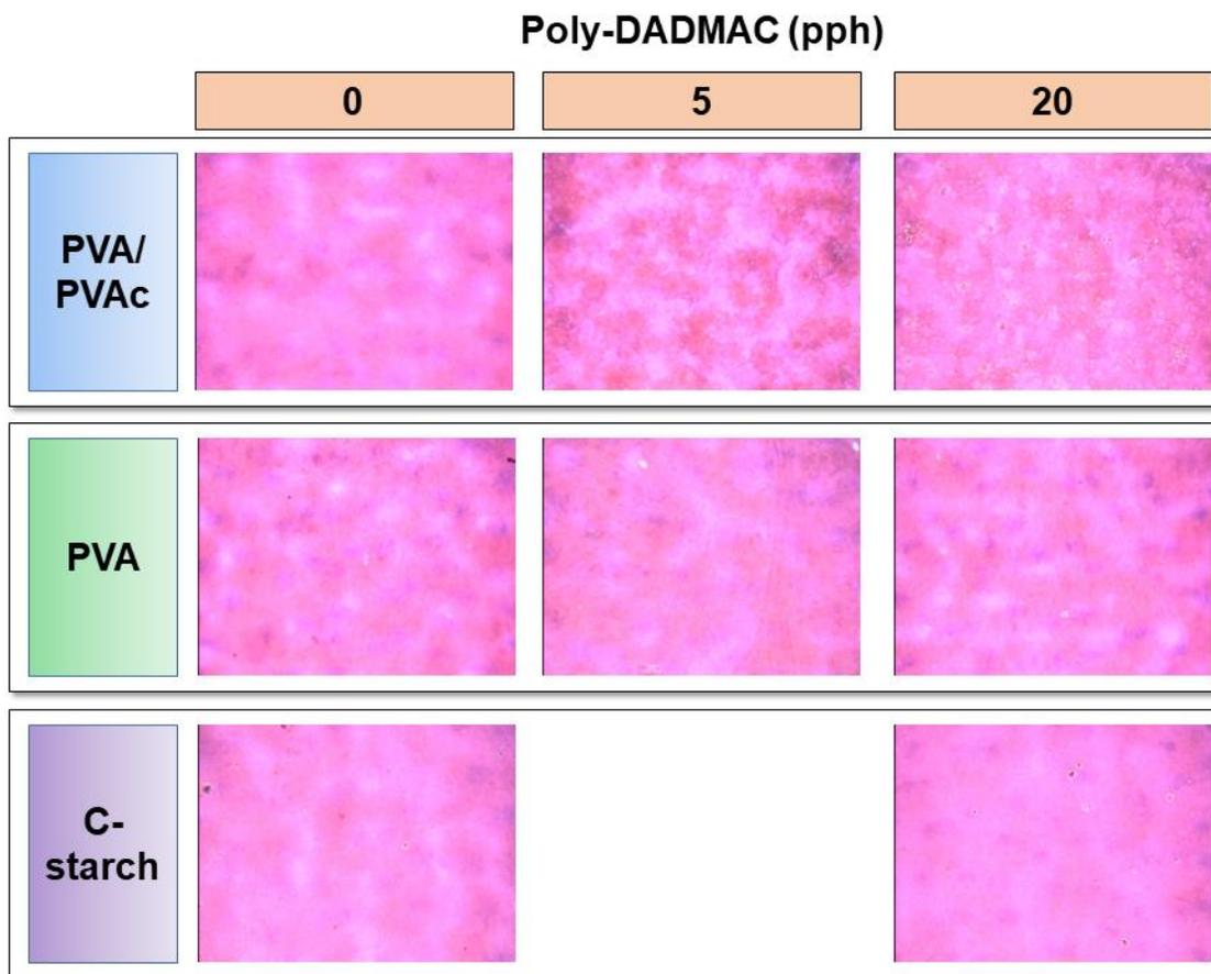
**Fig. 8.** Optical microscopy images (x400) of printed binder films with a dye-based ink
