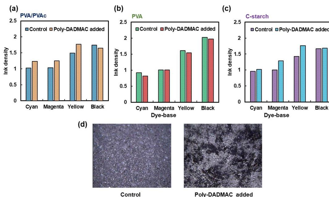
**Fig. 9.** The ink density of the coated paper after printing. The densitometer results of coated paper consisting of (a) PVA/PVAc, (b) PVA, and (c) C-starch binder system; and (d) optical microscopy images (x400) of printed coated paper consisting of PVA/PVAc binder system (Note: the cyan, magenta, and yellow inks are dye-based and black ink is pigment-based)
