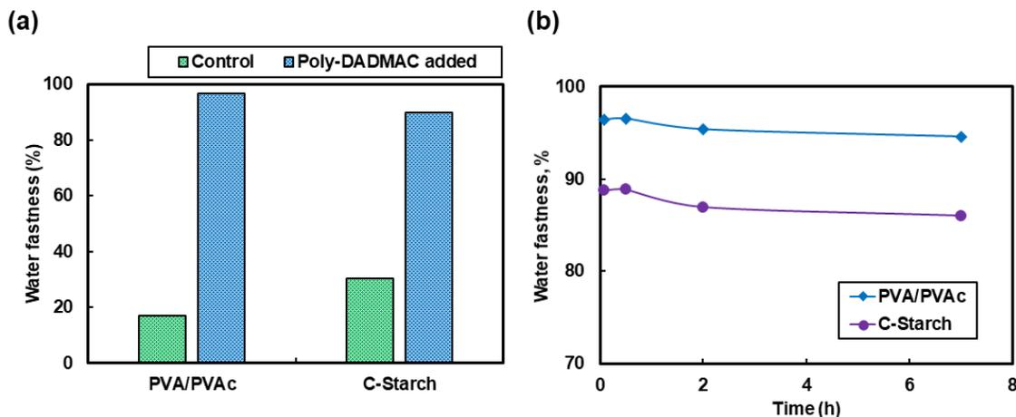
**Fig. 10.** The water fastness of coated paper after printing (dye-based ink): (a) water fastness of coated papers after 5 min of immersion to water; and (b) time dependent water fastness after the addition of poly-DADMAC
