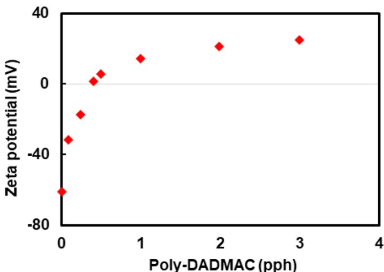
**Fig. 3.** Zeta potential of the silica suspension with the addition of poly-DADMAC
