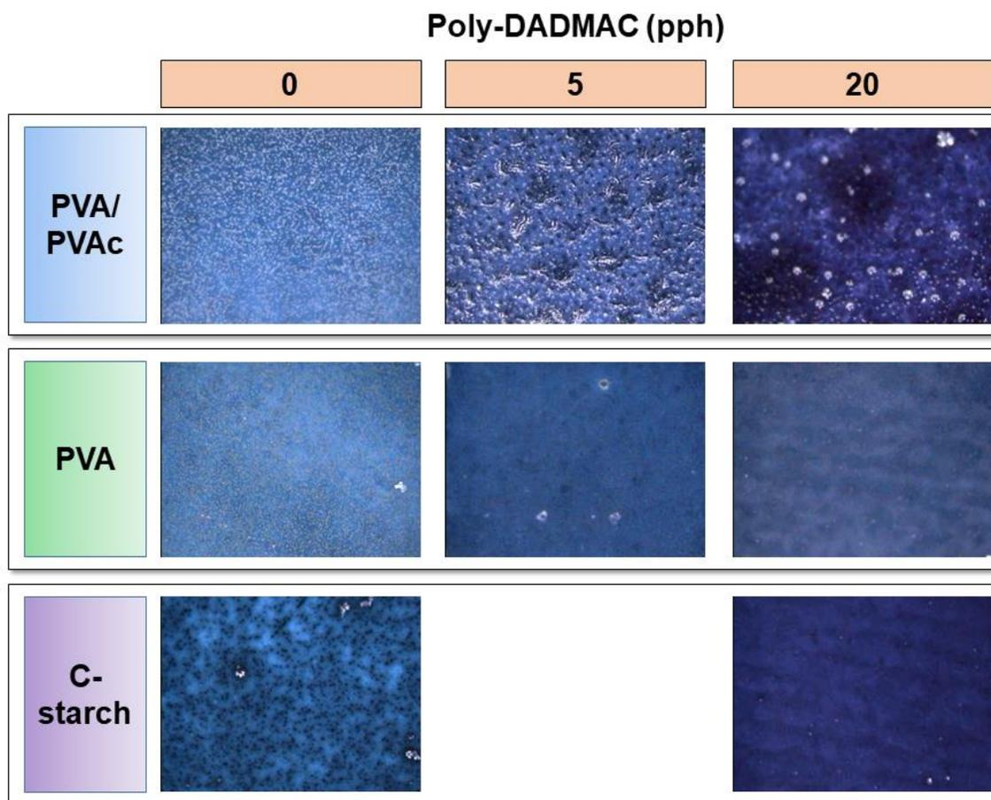
**Fig. 6.** Optical microscope images (x400) of printed binder films (pigment-based ink)
