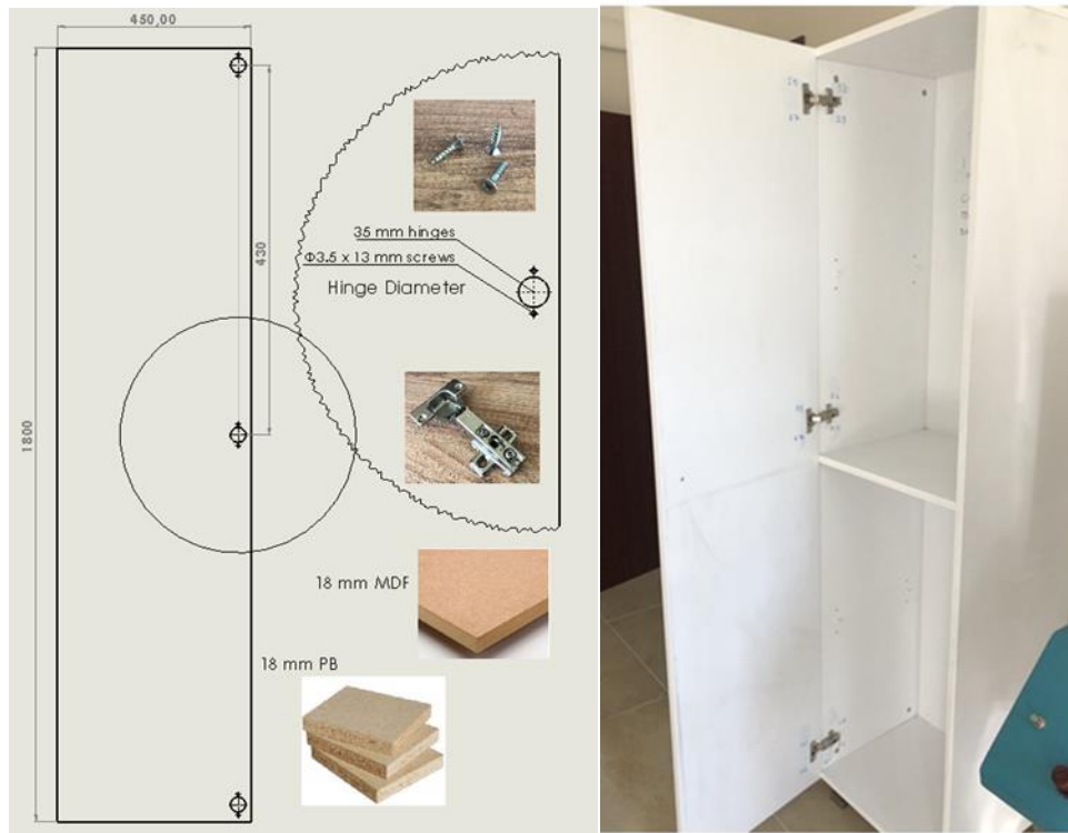
Fig. 1. Dimensions of samples and mounting holes; hinges
