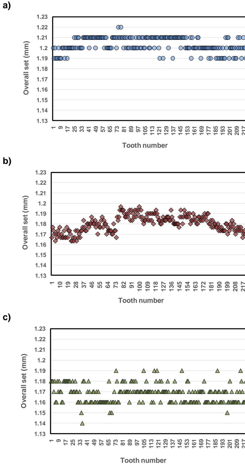
**Fig. 2.** Overall sets of band saws, where: new band saw (a), after re-sawing process while tool life is achieved for test No 1 (b), and after re-sawing process when tool life is reached for test No 2 (c)
