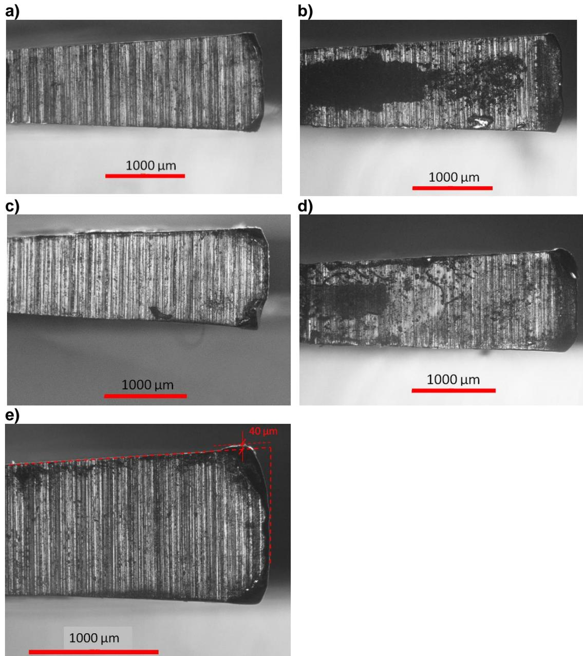
**Fig. 5.** Views in direction of clearance face  $A_\alpha$  of the tooth #202 (a), tooth #25 (c), and tooth #148 with dimensioned plastically deformed corner (f), and in direction of rake face  $A_\gamma$  of the tooth #202 (b), tooth #25 (d) (magnification of 2.5 $\times$ )
