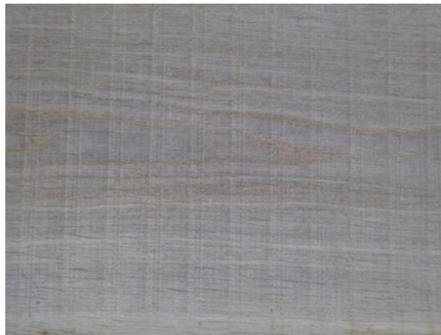
**Fig. 4.** Marks visible on the sawn surface of the oak lamella caused by the broken down tooth #143
