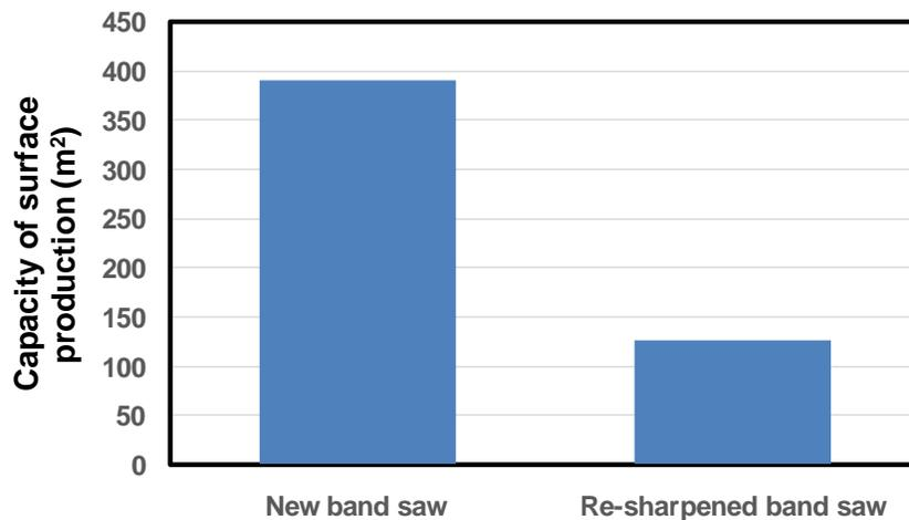
**Fig. 3.** Capacity of surface production as a function of band saw applied
