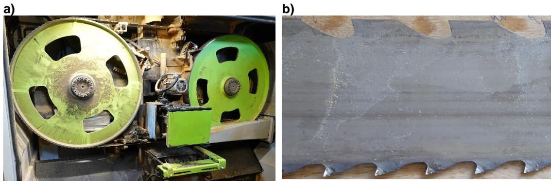
**Fig. 1.** General view of the working section of the band sawing machine DSB Singlehead NG XM (a), and a bandsaw with working (at the bottom) and scraper teeth (on the top) (b)
