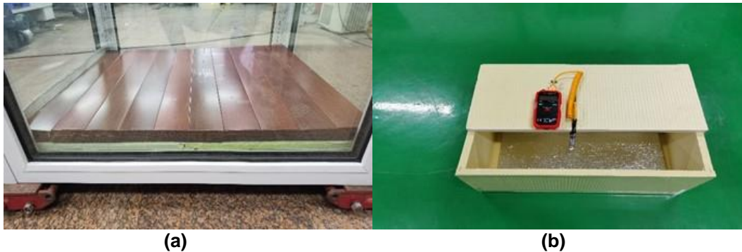
Fig. 8. Test piece of the floor (a); and test temperature measuring device (b)
