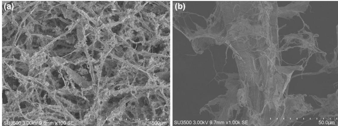
**Fig. 6.** SEM images of the morphological structure of fibres refined using refiner plates with circular bars; (a) – fibre overview; (b) – single fibre view
