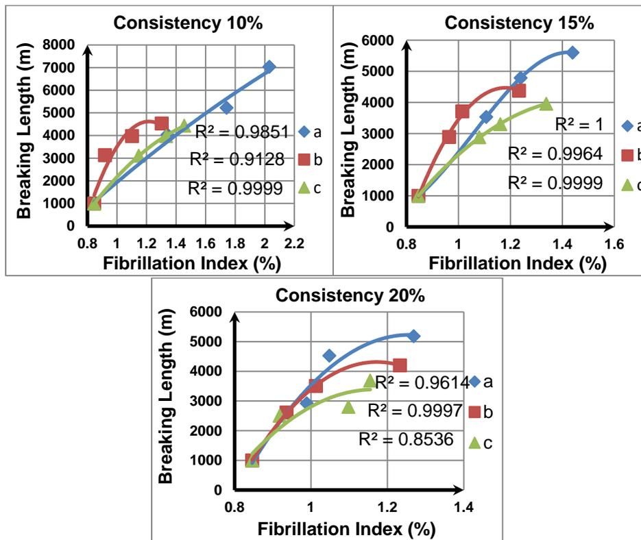
**Fig. 9.** Dependence of breaking length on the fibrillation index for different pulp consistencies and different refiner plate designs: (a) – with circular bars; (b) – sectoral with straight bars; (c) – with evenly distributed straight bars
