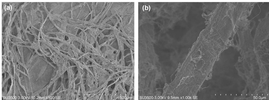
**Fig. 8.** SEM images of the morphological structure of fibres refined using refiner plates with evenly-distributed straight bars; (a) – fibre overview; (b) – single fibre view
