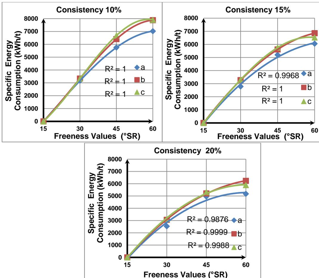
**Fig. 12.** Dependence of specific energy consumption on the freeness values for different pulp consistencies and different refiner plate designs: (a) – with circular bars; (b) – sectoral with straight bars; (c) – with evenly distributed straight bars
