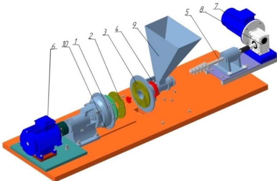
**Fig. 3.** Design of disc refiner (1 – refining zone; 2 – rotor; 3 – stator; 4 – adjusting device; 5 – screw feeder; 6 – rotor electric motor; 7 – screw feeder drive electric motor; 8 – worm gear; 9 – hopper; 10 – output)
