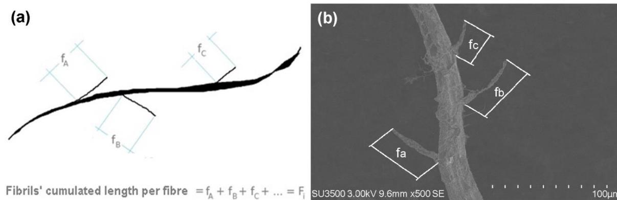
**Fig. 4.** Identification of the external fibrils: (a) – using the fibre analyser; (b) – using scanning electron microscopy
