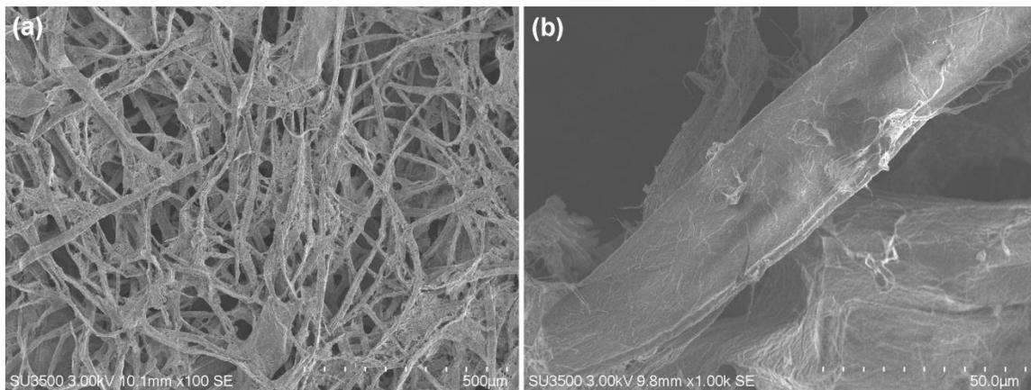
**Fig. 7.** SEM images of the morphological structure of fibres refined using sectoral refiner plates with straight bars; (a) – fibre overview; (b) – single fibre view
