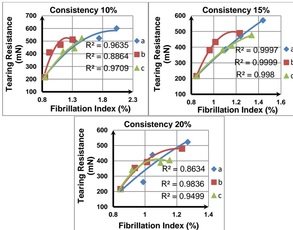
**Fig. 11.** Dependence of tear resistance on the fibrillation index for different pulp consistencies and different refiner plate designs: (a) – with circular bars; (b) – sectoral with straight bars; (c) – with evenly distributed straight bars
