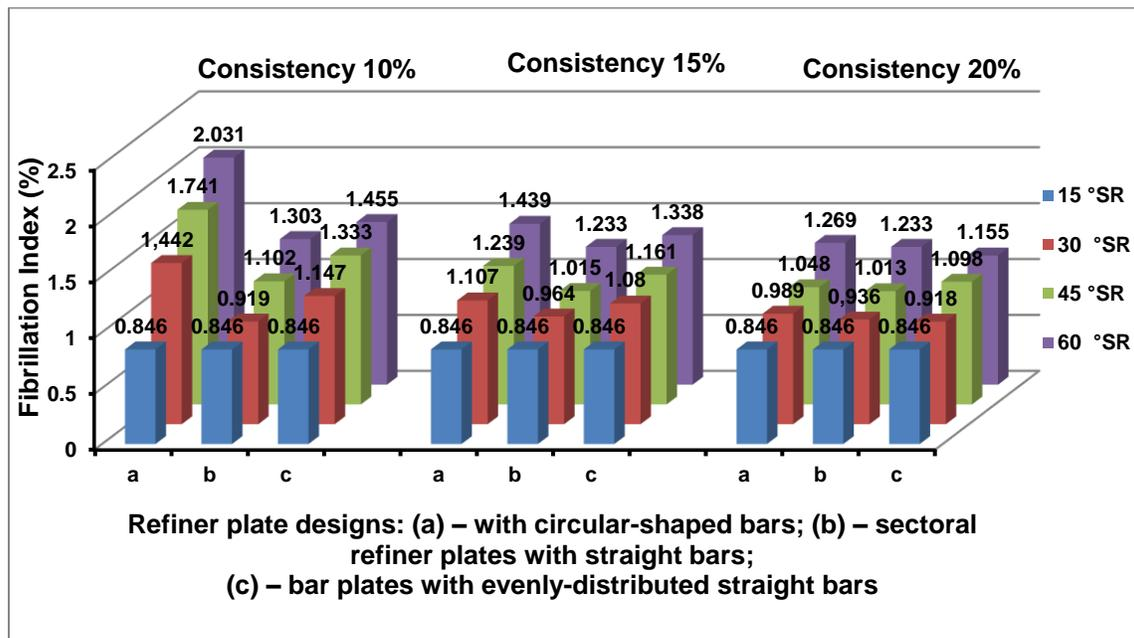
**Fig. 5.** Dependence of the fibrillation index on the freeness value for pulps of various consistency using different refiner plate designs
