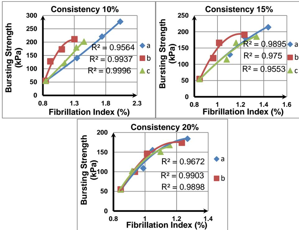
**Fig. 10.** Dependence of bursting strength on the fibrillation index for different pulp consistencies and different refiner plate designs: (a) – with circular bars; (b) – sectoral with straight bars; (c) – with evenly distributed straight bars
