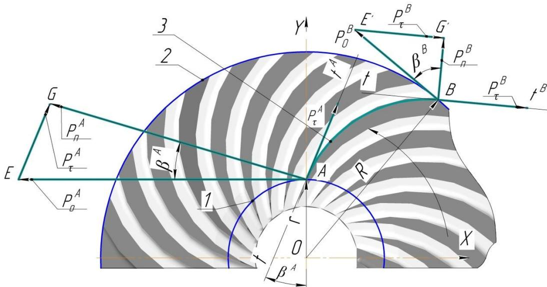
**Fig. 2.** Fragment of the rotor disc refiner plate with the force components of the circular bar
