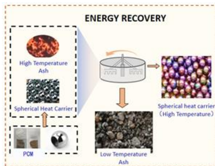
Fig. 4. The system of recovering heat energy by phase-change heat carrier
