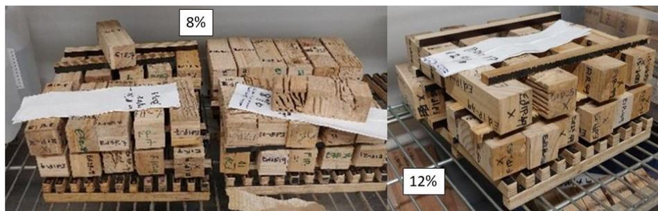
**Fig. 4.** Harvested and cleaned samples placed in the conditioning chamber at 12% and 8% MC before any further measurement and analysis
