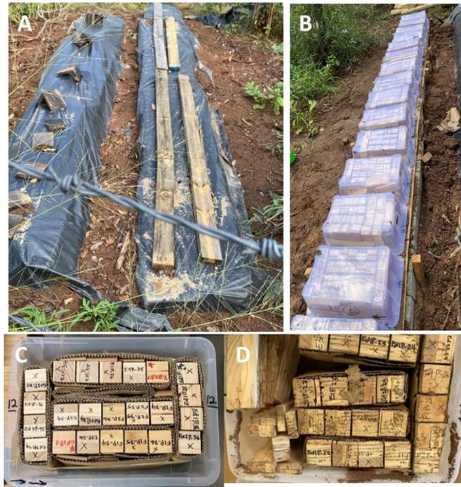
**Fig. 3.** (A) Trench used for exposing samples to termite foraging, (B) sample boxes placed in the trench for the period of exposure to termite foraging, (C) samples packed in cardboard sections and placed in boxes to be exposed to termite attack, and (D) harvested sample box after termite exposure
