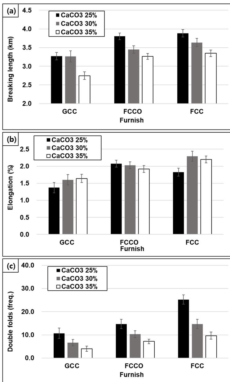
**Fig. 6.** Breaking length (a), elongation at break (b), and folding property (c) of the papers containing different fillers
