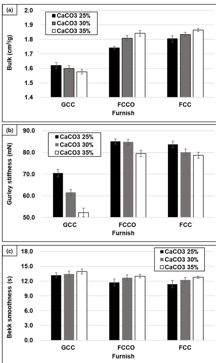
**Fig. 5.** Bulk (a), Gurley stiffness (b), and Bekk smoothness (c) of the papers containing three different fillers
