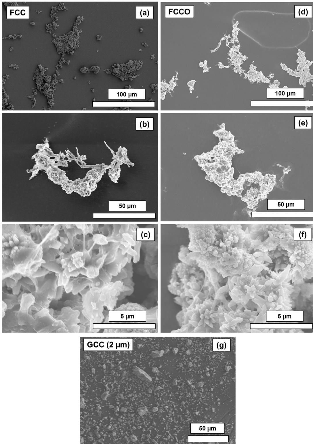
**Fig. 2.** Micrographs of flexible calcium carbonate from MFC (FCC, a to c), and MFCO (FCCO, d to f), and GCC (g). The images (b), (e) and (c), (f) are high magnification of 1K, and 10K, respectively for each FCC.
