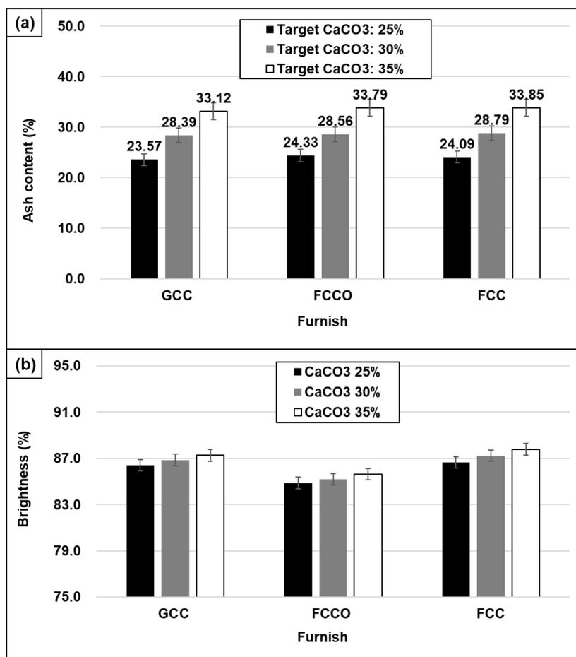
Fig. 3. Ash content (a) and brightness (b) of the papers containing three different fillers
