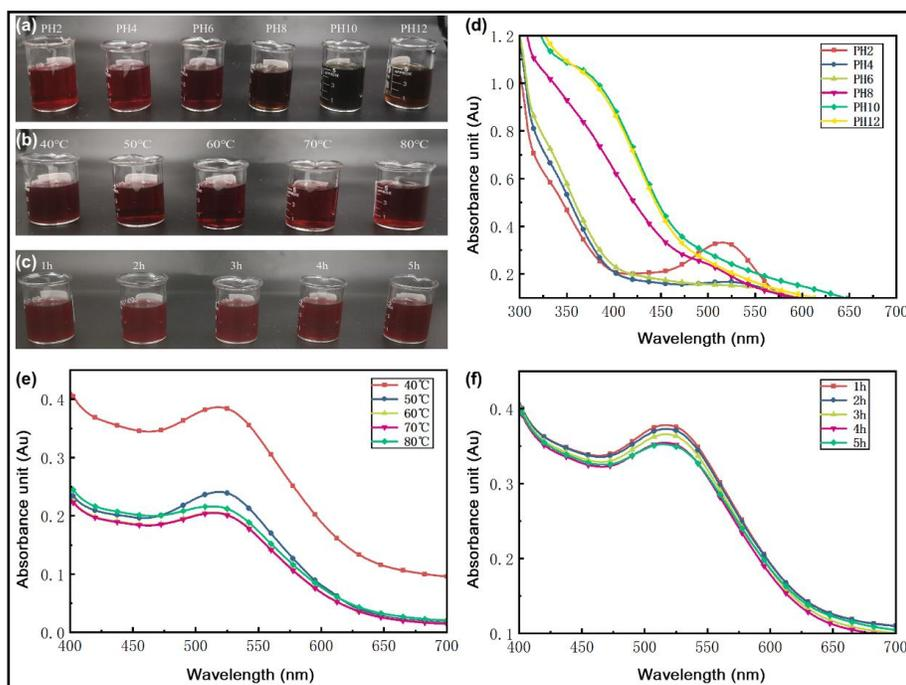
**Fig. 7.** Digital images of the effect of (a) pH, (b) temperature, and (c) UV irradiation on *Cinnamomum camphora* fruit dye; (d) UV spectra of the effect of pH on the absorbance, (e) UV spectra of the effect of temperature on the absorbance, and (f) UV spectra of the effect of UV irradiation on the absorbance of *Cinnamomum camphora* fruit dye
