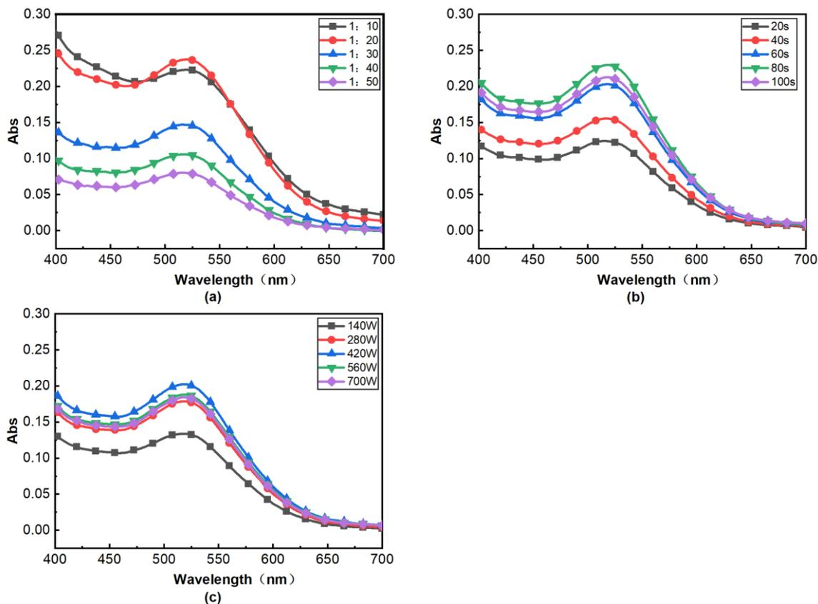
**Fig. 1.** (a)The influence of solid-liquid ratio on dye absorbance, (b)The influence of microwave time on dye absorbance, and (c)The influence of microwave power on dye absorbance
