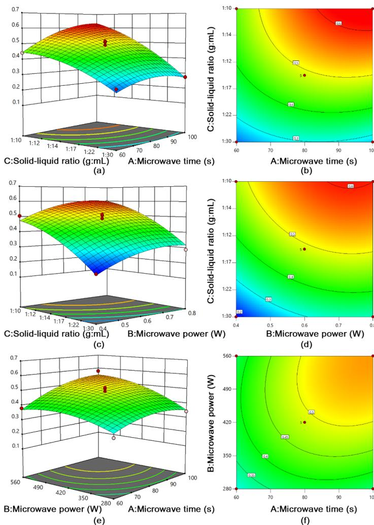
**Fig. 3.** Response surface plot (a) and contour plot (b) of the ratio and microwave time on the absorbance; Response surface plot (c) and contour plot (d) of the absorbance by the ratio of liquid to microwave power; Response surface plot (e) and contour plot (f) of microwave power versus microwave time on the absorbance during *Cinnamomum camphora* fruit dye extraction
