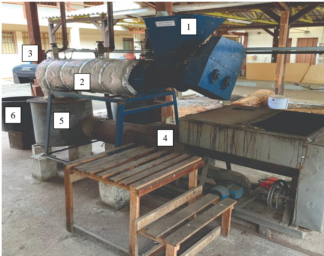
Fig. 1. Lateral view of the screw reactor for thermal treatment of lignocellulosic biomass: 1 - input biomass; 2 - heating system; 3 - cooling system; 4 – burner; 5 - connection chimney with the burner; 6 - torrefied biomass exit
