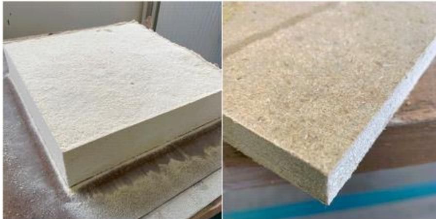
**Fig. 1.** The homogenised mixture after pre-forming (left) and the composite board after pressing (right)
