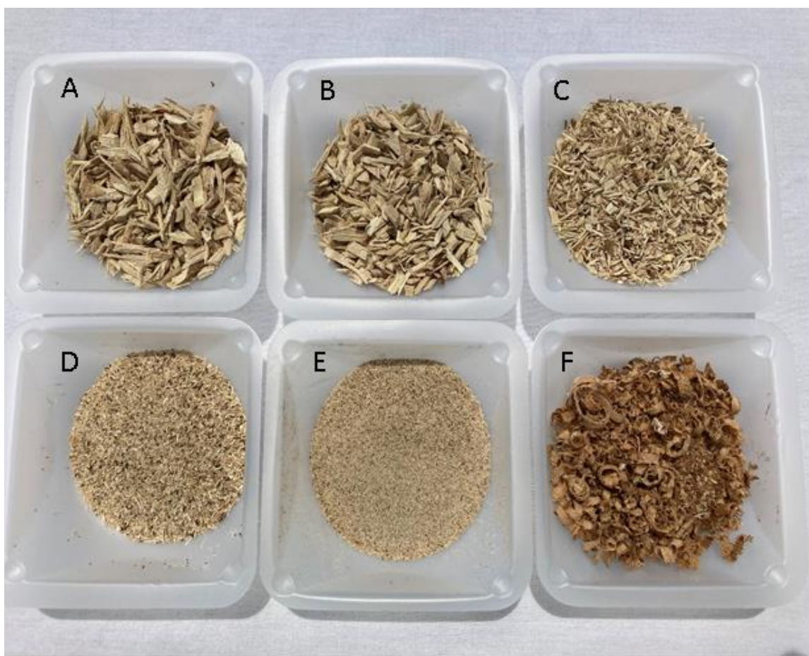
Fig. 5. Frost grape stem chips after milling and fractionating with sieves (A-E) and scraped frost grape stem inner bark (F). For scale, plastic weigh trays are 8.7 cm wide.
