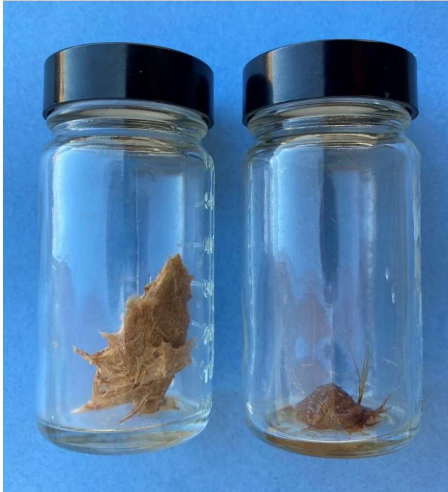
Fig. 6. Two examples of freeze-dried frost grape stem chip extract samples inadequately protected against humid laboratory conditions showing varying degrees of darkening and decreased volume
