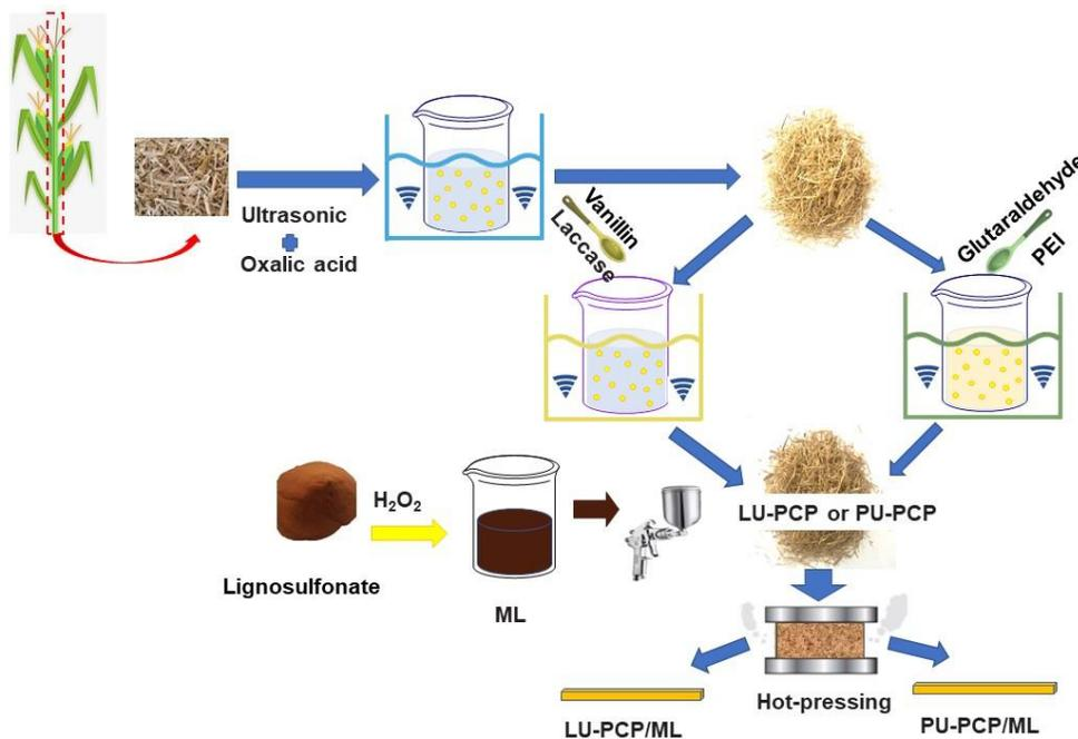
**Fig. 1.** Schematic illustration of fabrication processes of the LU-PCP/ML and PU-PCP/ML composites
