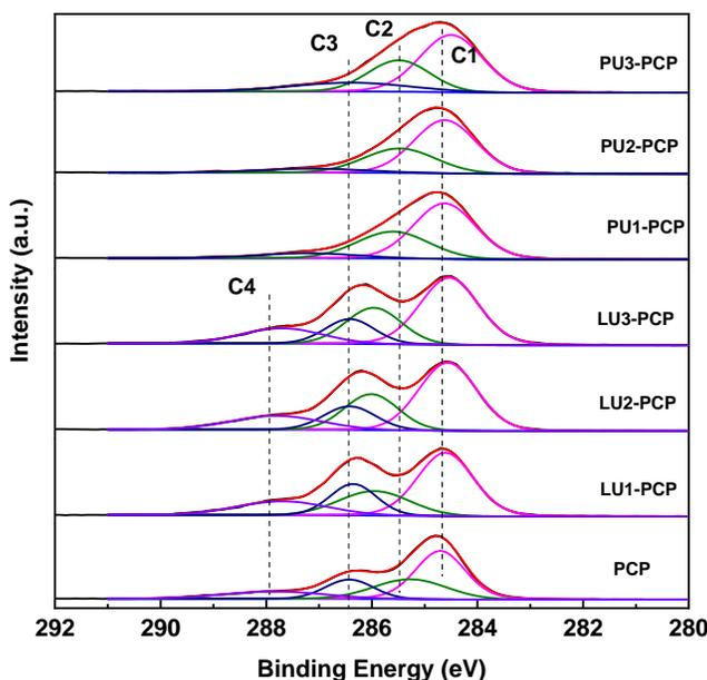
**Fig. 3.** XPS C 1s spectra of PCP after different modified treatments
