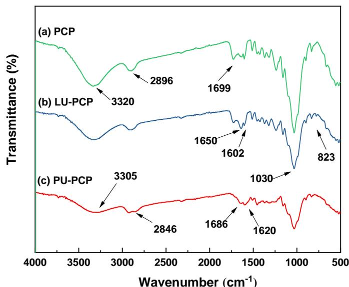
**Fig. 2.** FTIR spectra of the (a) as-prepared PCP and PCP treated with (b) laccase (85 U/g-PCP) and (c) PEI (2 wt%)
