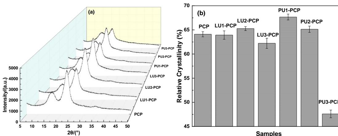
**Fig. 4.** XRD patterns and relative crystallinity of PCP after different modified treatments
