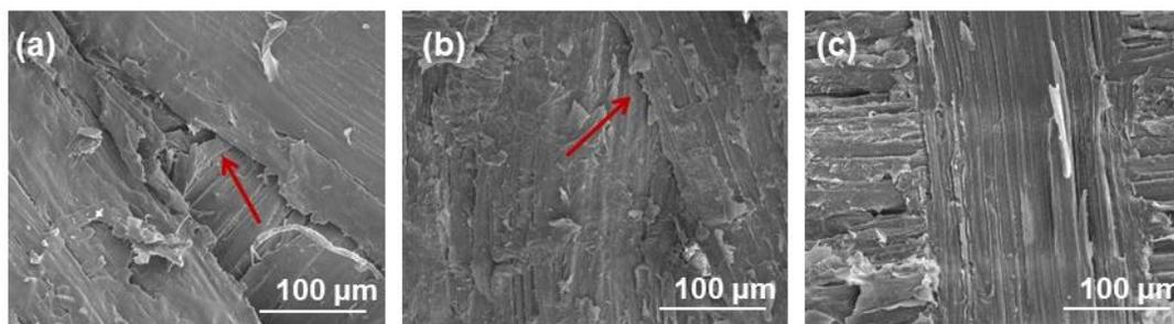
**Fig. 6.** The peeling surfaces of (a) PCP/ML, (b) LU-PCP/ML, and (c) PU-PCP/ML composites
