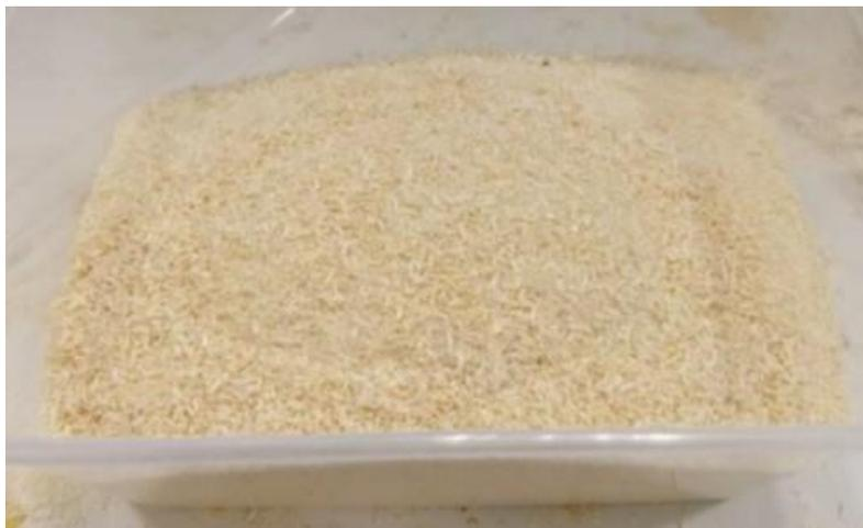
**Fig. 1.** The sieved ground pine particles
