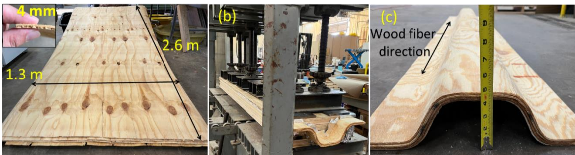
Fig. 3. Manufacturing process; (a) full-size, veneers with defects having an average thickness of 4 mm and (b) cold-pressing of four veneers to fabricate (c) Final corrugated panels with 432mm-wide and 2.6m-long dimensions
