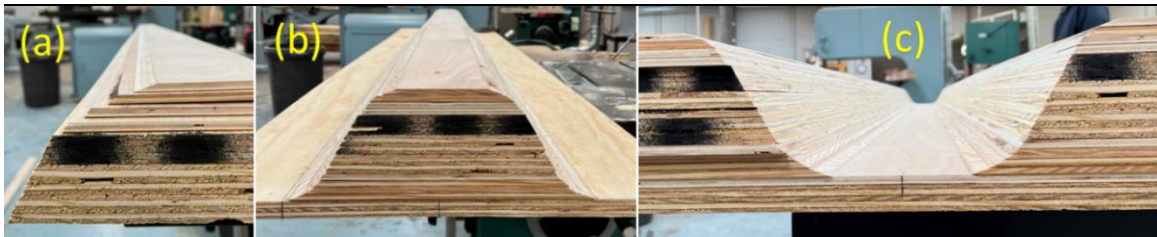
Fig. 2. (a) Cutting veneer in size and angle, (b) upper part (male) and (c) lower part (female) of the wooden mold with rounded corners
