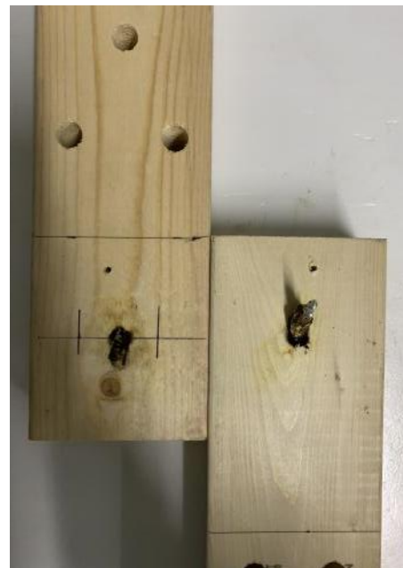
Fig. 5. Failure pattern of composite dowel joint member
