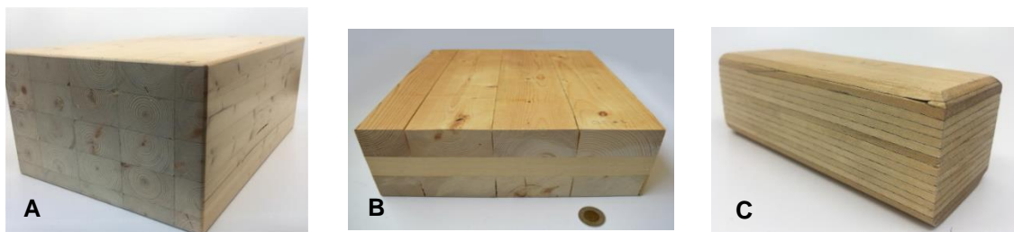
Fig. 1. Structural wood products evaluated in this study: A) Glued laminated timber (GLT), B) cross laminated timber (CLT) and C) laminated veneer lumber (LVL)
