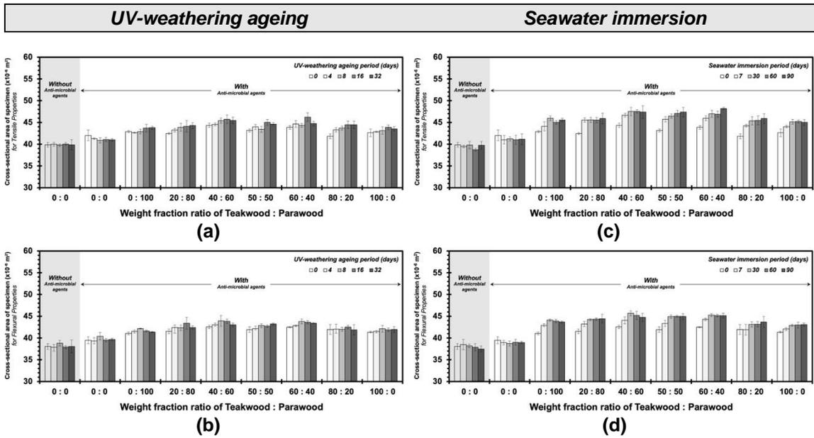
Fig. 1. The cross-sectional area of the specimens for (a), (c) tensile and (b), (d) flexural tests as a function of UV-weathering ageing and seawater immersion periods
