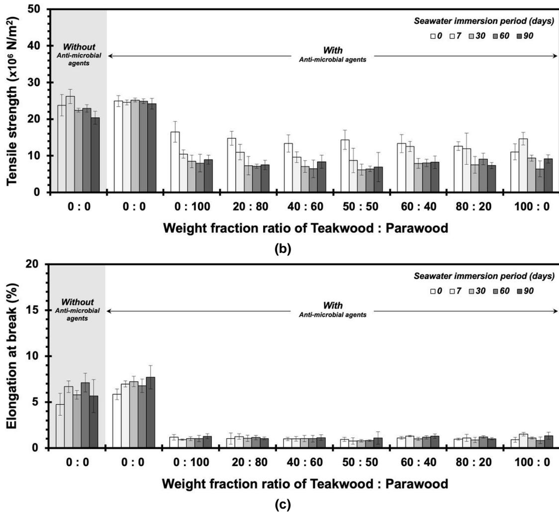
**Fig. 6.** (a) Tensile modulus, (b) strength, and (c) elongation at break as a function of seawater immersion periods
