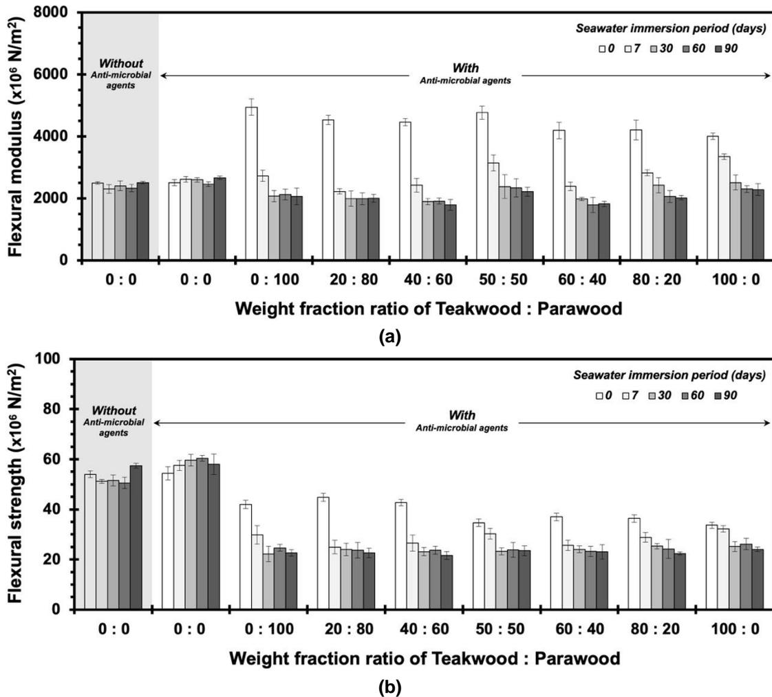
Fig. 7. (a) Flexural modulus and (b) strength as a function of seawater immersion periods
