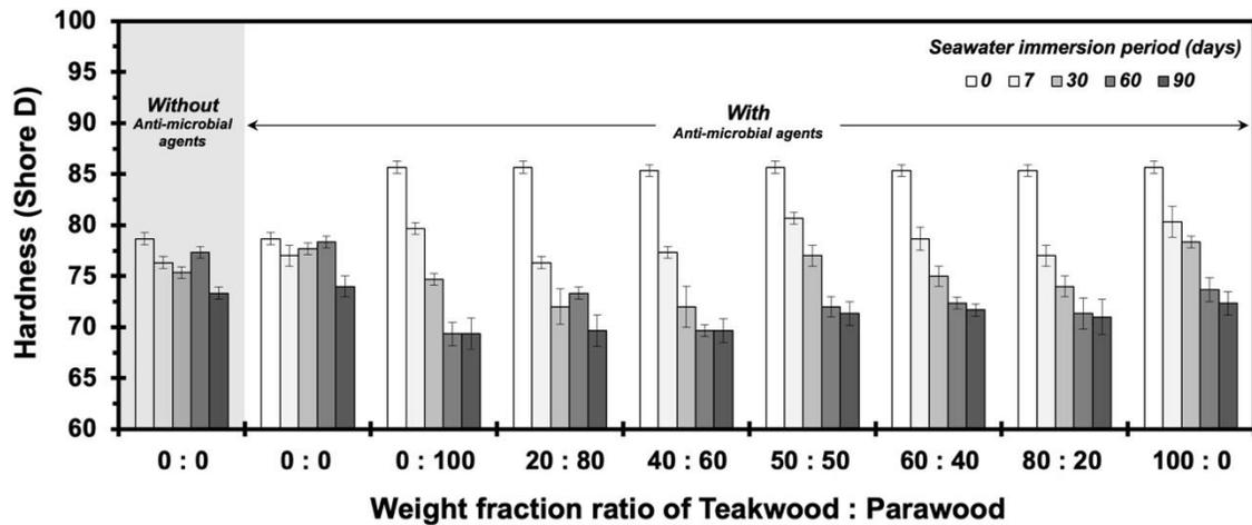
Fig. 8. The hardness of the specimens as a function of seawater immersion periods
