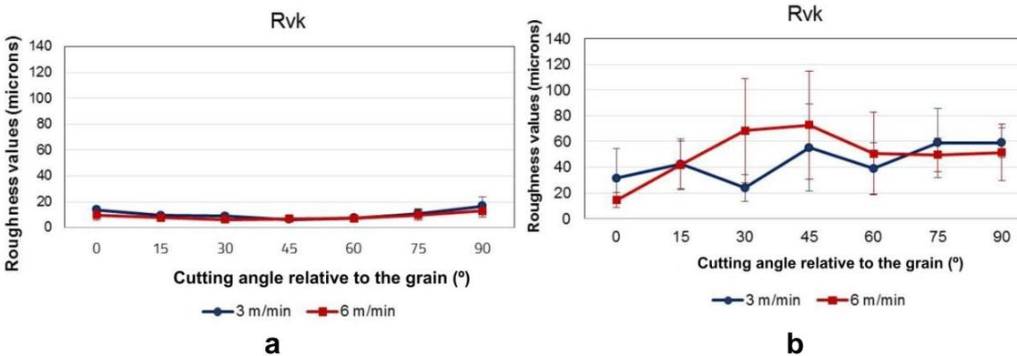
**Fig. 11.** The mean values of the  $R_{vk}$  parameter, CNC routed with two feed speeds and seven cutting angles as function of grain orientation: (a) maple surface; (b) oak surface
