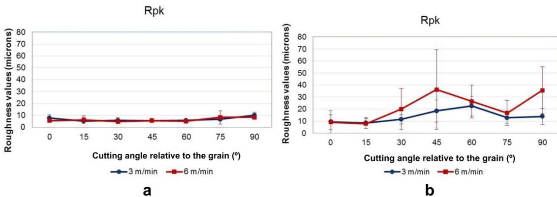
**Fig. 8.** The mean values of the  $R_{pk}$  parameter, CNC routed with two feed speeds and seven cutting angles as function of grain orientation: (a) maple surface; (b) oak surface
