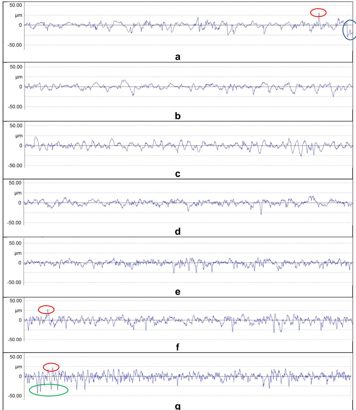
**Fig. 4.** Roughness profiles of maple, for  $u=3$  m/min for various cutting angles as related to the grain: (a)  $0^\circ$ ; (b)  $15^\circ$ ; (c)  $30^\circ$ ; (d)  $45^\circ$ ; (e)  $60^\circ$ ; (f)  $75^\circ$ ; (g)  $90^\circ$ . Example of raised fiber is encircled with red, wood pores are encircled with green, and blue represents longitudinally cut pore.
