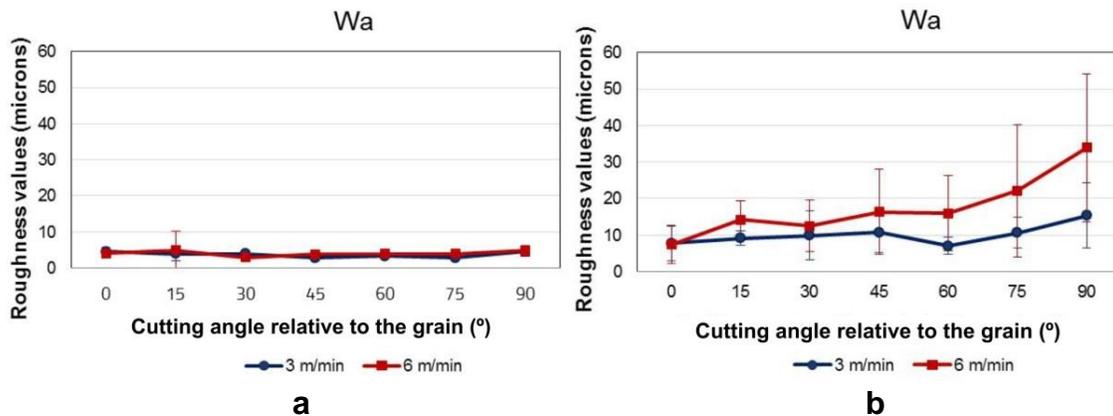
**Fig. 12.** The mean values of the  $W_a$  parameter, CNC routed with two feed speeds and seven cutting angles with relate to the grain; (a) evaluated for maple wood surface; (b) evaluated for oak wood surface
