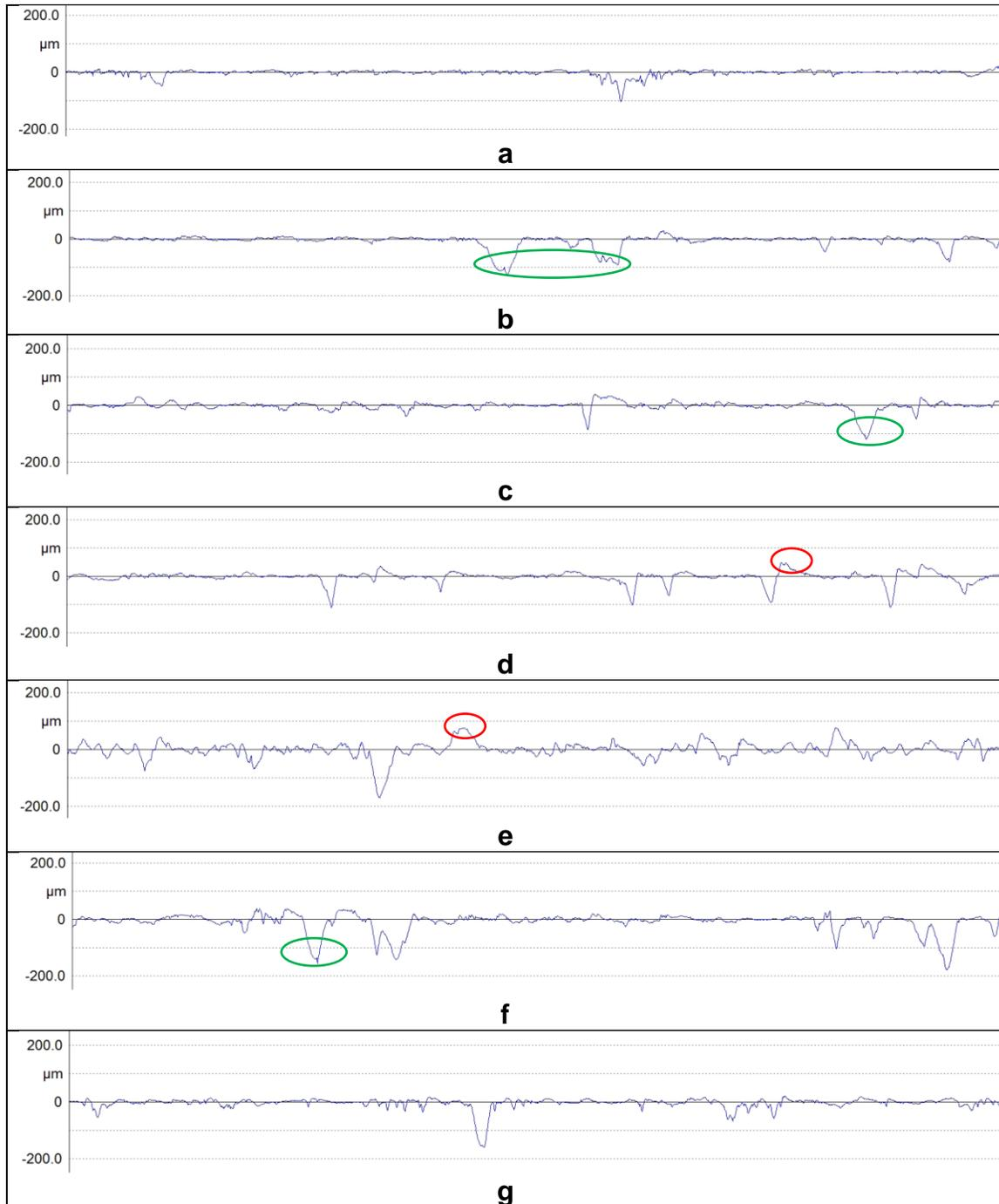
**Fig. 5.** Roughness profiles of oak, for  $u=3$  m/min for various cutting angles as related to the grain: (a)  $0^\circ$ ; (b)  $15^\circ$ ; (c)  $30^\circ$ ; (d)  $45^\circ$ ; (e)  $60^\circ$ ; (f)  $75^\circ$ ; (g)  $90^\circ$ . Examples of raised fiber are encircled with red and wood pores are encircled with green.
