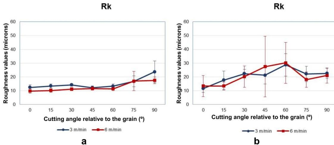
**Fig. 6.** The mean values of the core roughness,  $R_k$ , CNC routed with two feed speeds and seven cutting angles with relate to the grain: (a) evaluated for maple surface; (b) evaluated for oak surface
