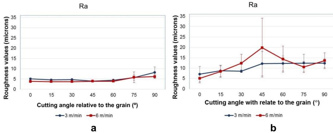
**Fig. 7.** The mean values of the  $R_a$  parameter, CNC routed with two feed speeds and seven cutting angles as function of the grain orientation: (a) evaluated for maple surface; (b) evaluated for oak surface
