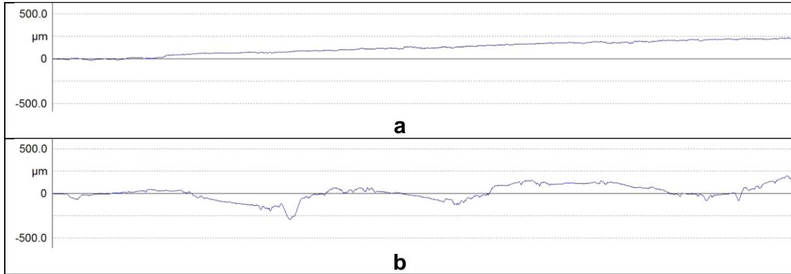
**Fig. 13.** Comparative surface profiles of oak sample, containing roughness and waviness together from surfaces processed with  $u=6$  m/min: (a) cutting along the grain orientation; (b) cutting at  $90^\circ$  as related to the grain
