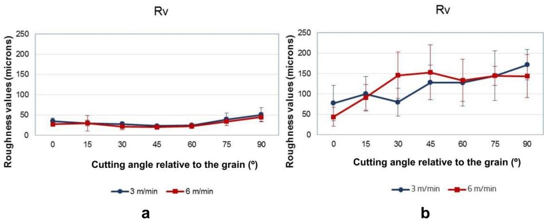
**Fig. 10.** The mean values of the  $R_v$  parameter, CNC routed with two feed speeds and seven cutting angles as function of grain orientation: (a) maple surface; (b) oak surface
