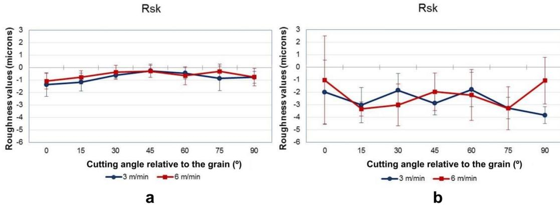
**Fig. 9.** The mean values of the  $R_{sk}$  parameter, CNC routed with two feed speeds and seven cutting angles as function of grain orientation: (a) maple surface; (b) oak surface
