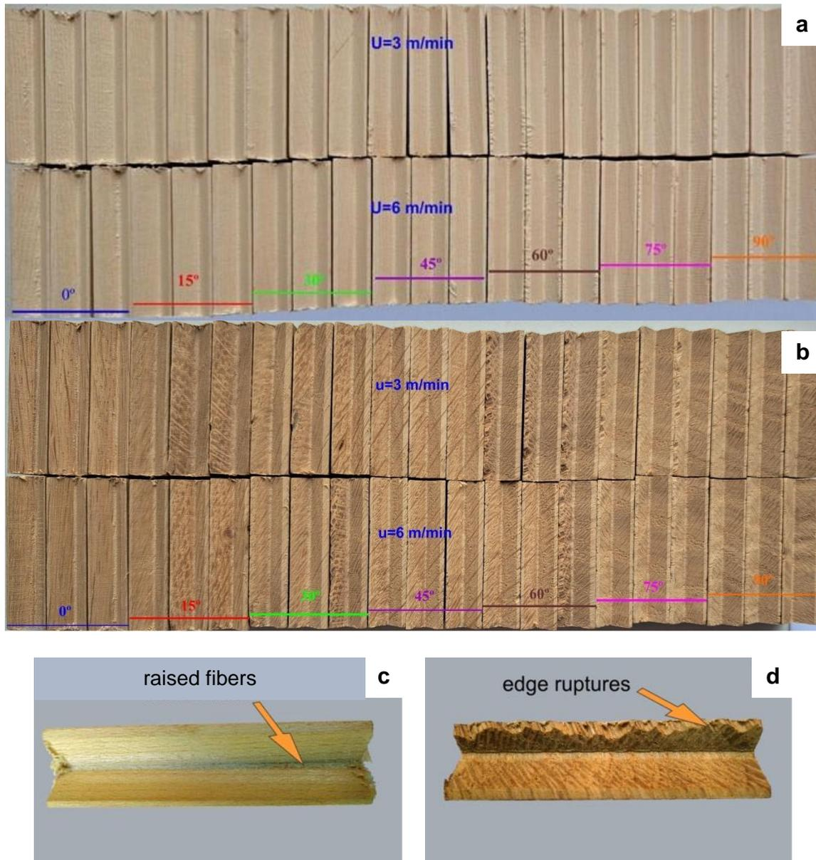
Fig. 3. Roughness measurements of maple (a, c) and oak (b, d) samples
