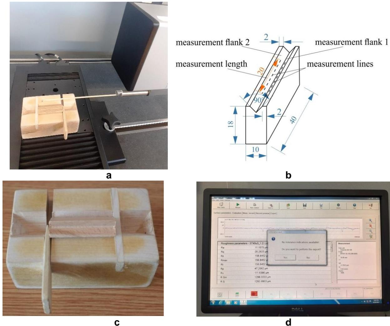
**Fig. 2.** MarSurf XT20 profilometer used to measure the roughness and the holder used to position the measured surface perpendicular to the stylus direction: (a) stylus scanning the sample; (b) the sample with measurements; (c) the specimen holder with the sample fixed on top; (d) screen displaying the measured parameters
