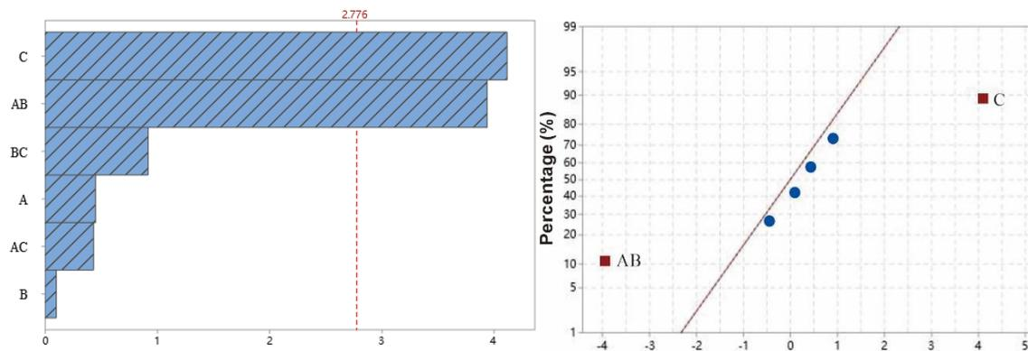
**Fig. 5.** Pareto plot and normal plot of standardized effects for moisture resistance modulus of rupture
