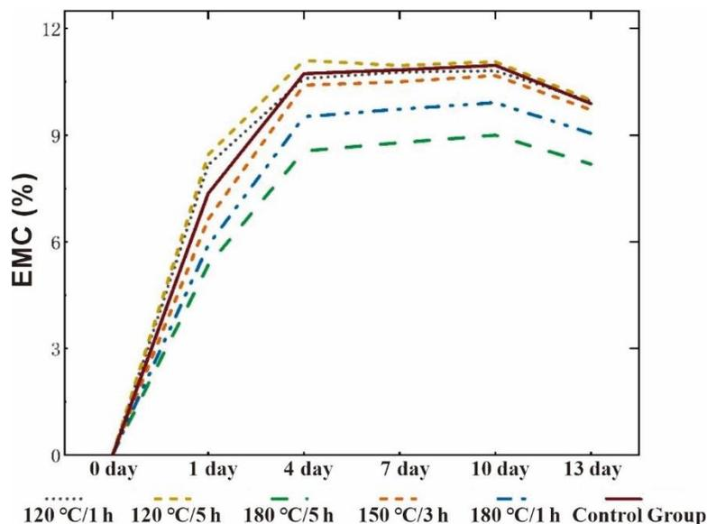
**Fig. 4.** Moisture sorption process of completely dry wood
