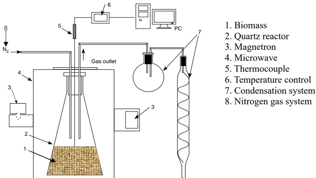
**Fig. 1.** Schematic of microwave heated torrefaction system
