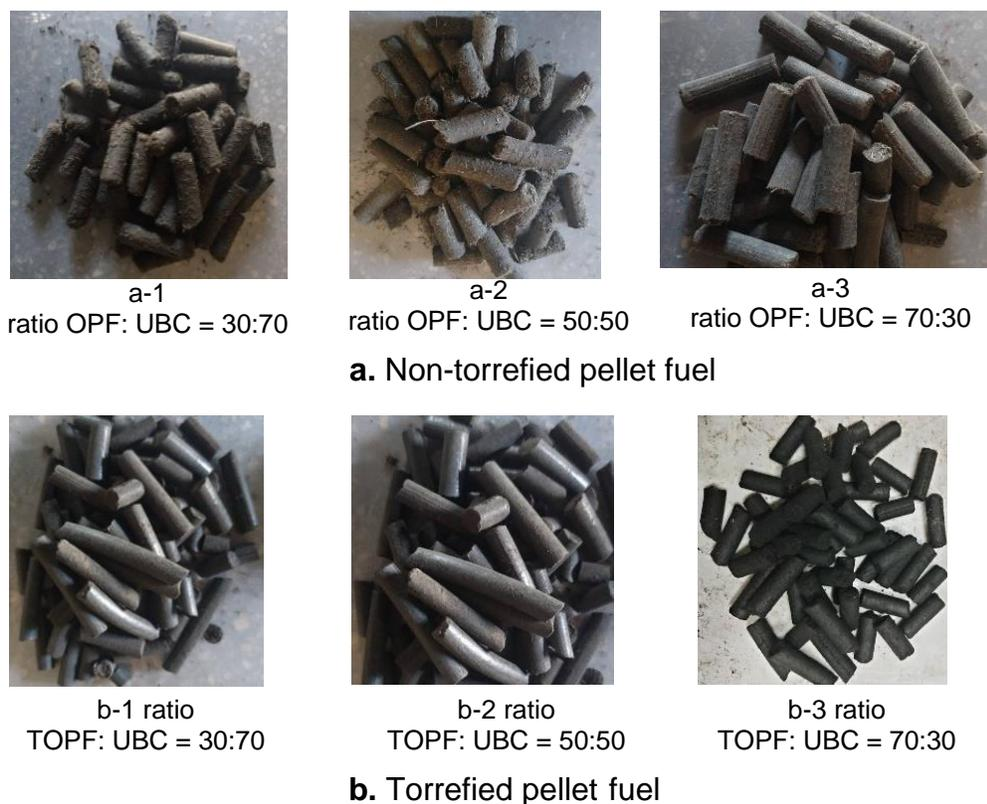
**Fig. 6.** Appearances of pellet fuels made with raw or torrefied biomass mixed with UBC
