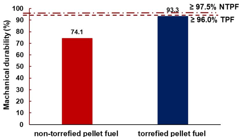
**Fig. 11.** Mechanical durability index of pellet fuels made with raw or torrefied biomass
