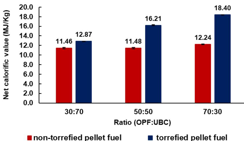
**Fig. 7.** Net calorific value of pellet fuels made with raw or torrefied biomass
