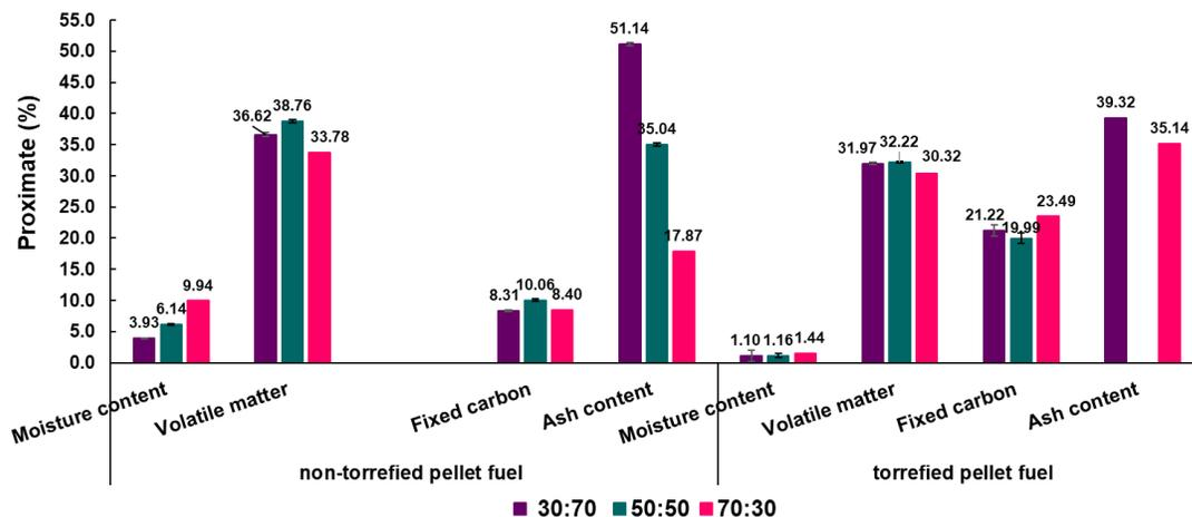
Fig. 8. Proximate analyses of pellet fuels made with raw and torrefied biomass
