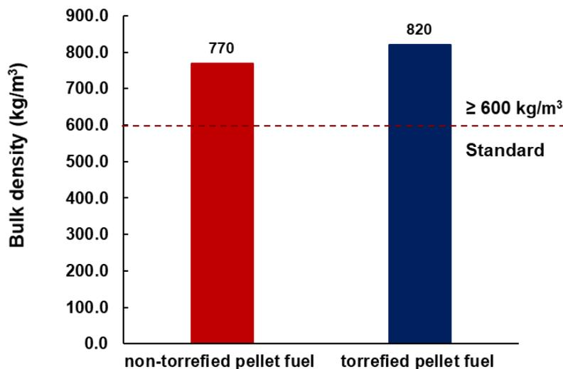
**Fig. 10.** Bulk density of pellet fuels made with raw or torrefied biomass
