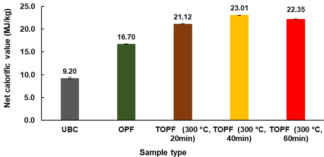
Fig. 3. Net calorific value of raw materials and torrefied oil palm frond
