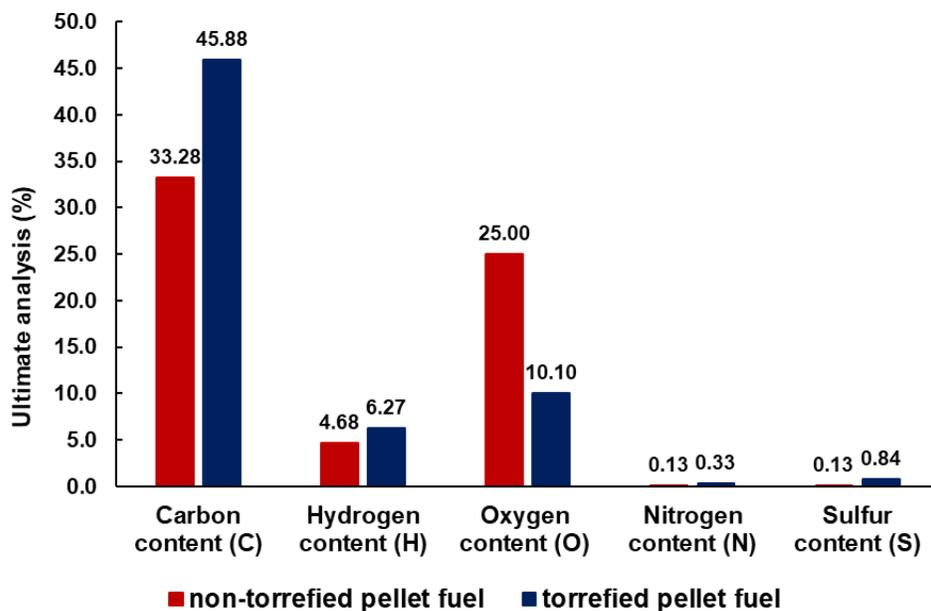
**Fig. 9.** Ultimate analyses of pellet fuels made with raw or torrefied biomass
