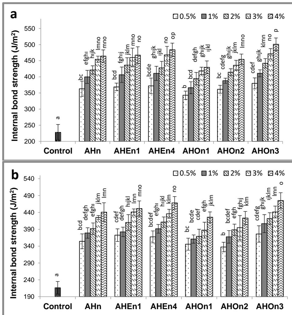
**Fig. 6.** The effect of starch/NFC suspensions on the internal bond strength of (a) fluting and (b) coreboard papers. Factors followed by the same letter were not significantly different (Duncan test at  $p < 0.05$ ).
