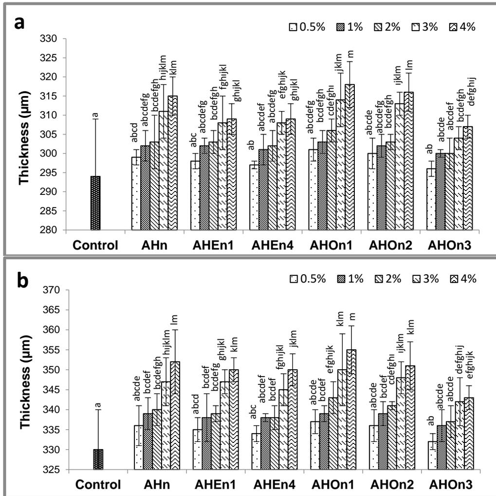
**Fig. 1.** The effect of starch/NFC suspensions on the thicknesses of (a) fluting and (b) coreboard papers. Factors followed by the same letter were not significantly different (Duncan test at  $p < 0.05$ ).
