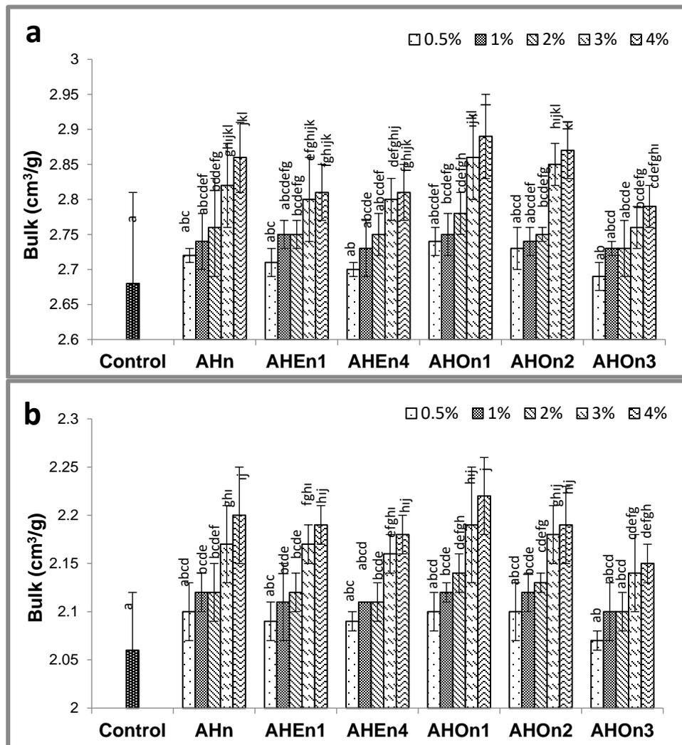
**Fig. 2.** The effect of starch/NFC suspensions on the bulk of (a) fluting and (b) coreboard papers. Factors followed by the same letter were not significantly different (Duncan test at  $p < 0.05$ ).
