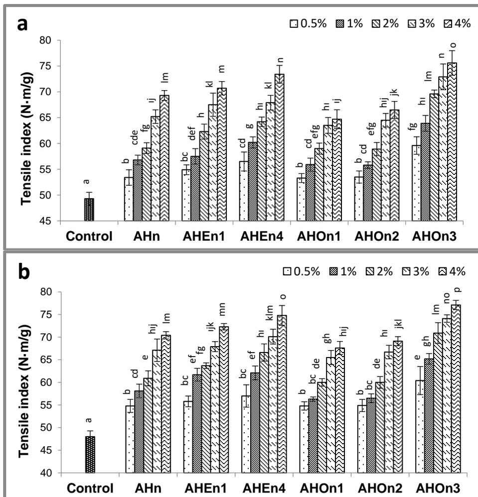
**Fig. 4.** The effect of starch/NFC suspensions on the tensile indices of (a) fluting and (b) coreboard papers. Factors followed by the same letter were not significantly different (Duncan test at  $p < 0.05$ ).
