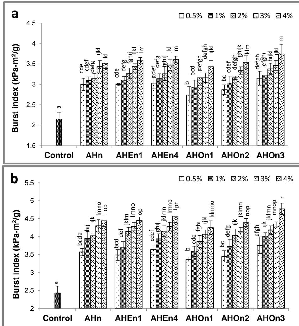
**Fig. 5.** The effect of starch/NFC suspensions on the burst indices of (a) fluting and (b) coreboard papers. Factors followed by the same letter were not significantly different (Duncan test at  $p < 0.05$ ).
