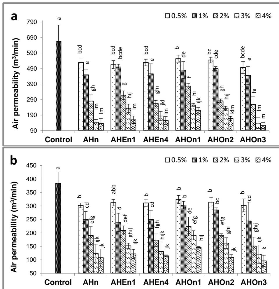
**Fig. 3.** The effect of starch/NFC suspensions on the air permeability of (a) fluting and (b) coreboard papers. Factors followed by the same letter were not significantly different (Duncan test at  $p < 0.05$ ).
