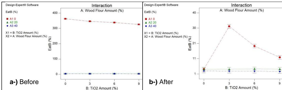
**Fig. 10.** The effects of fillers amount on elongation at break properties of WPCs: a-) Before weathering, b-) After weathering
