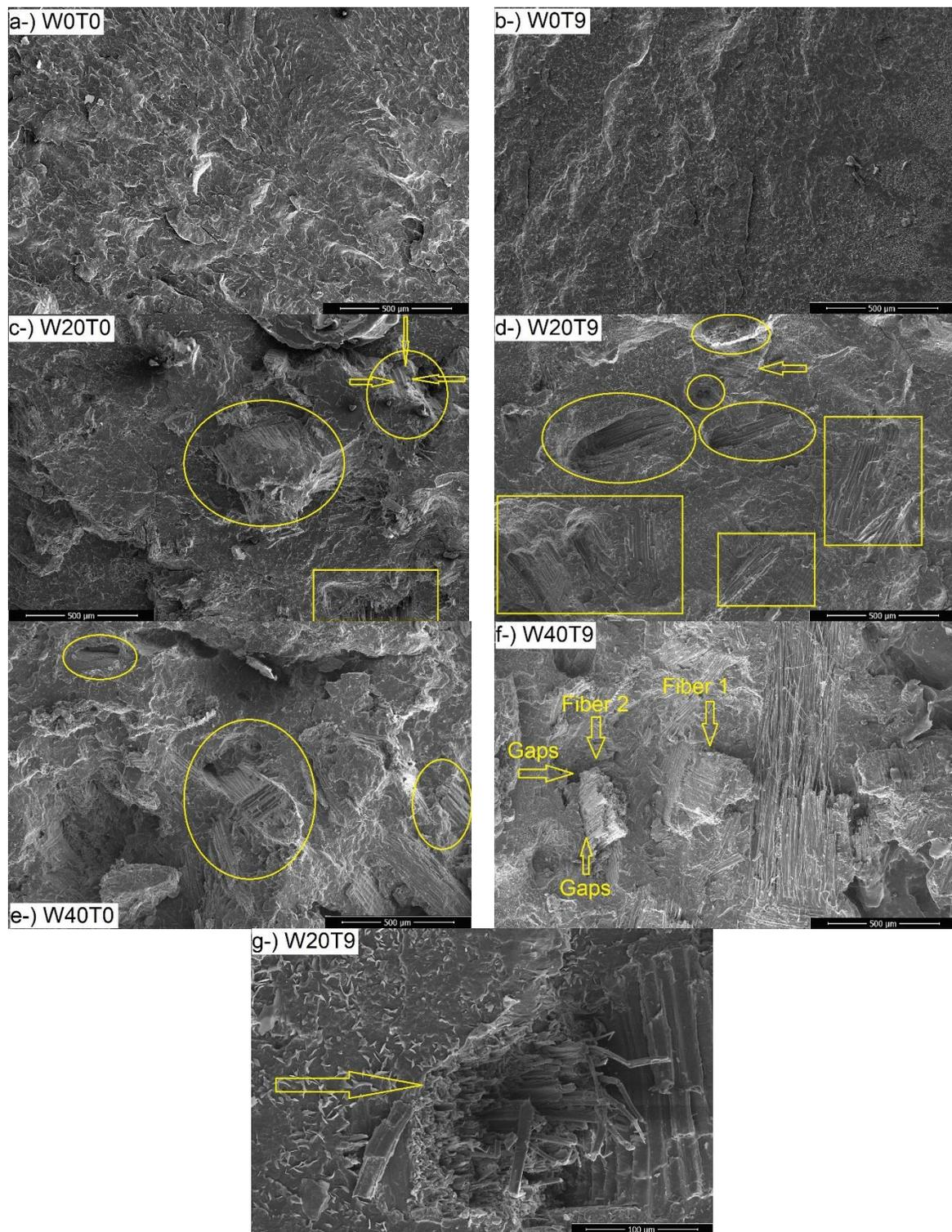
**Fig. 14.** SEM images (taken at 200 magnification, except g-) W20T0) of WPCs taken with a ETD detector; a-) W0T0, b-) W0T9, c-) W20T0, d-) W20T9, e-) W40T0, f-) W40T9, and g-) W20T9 (taken at 1000 magnification)
