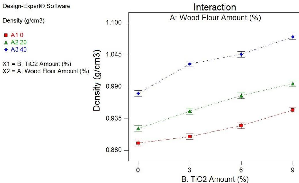
**Fig. 1.** WF and TiO<sub>2</sub> loadings effects on density of PP-based composites
