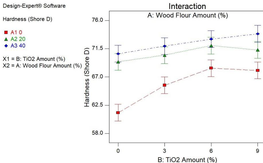
**Fig. 3.** WF and TiO<sub>2</sub> loadings effects on hardness of PP-based composites
