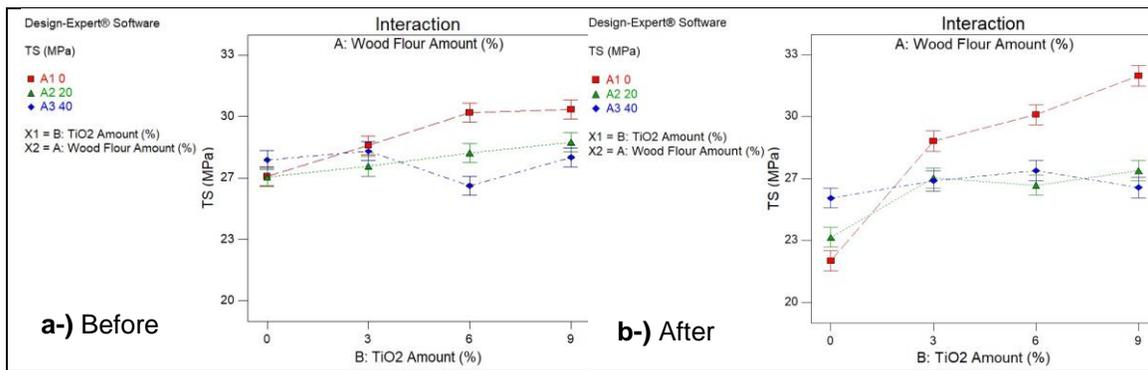
**Fig. 9.** The effects of fillers amount on tensile strength of WPCs; a-) Before weathering, b-) After weathering
