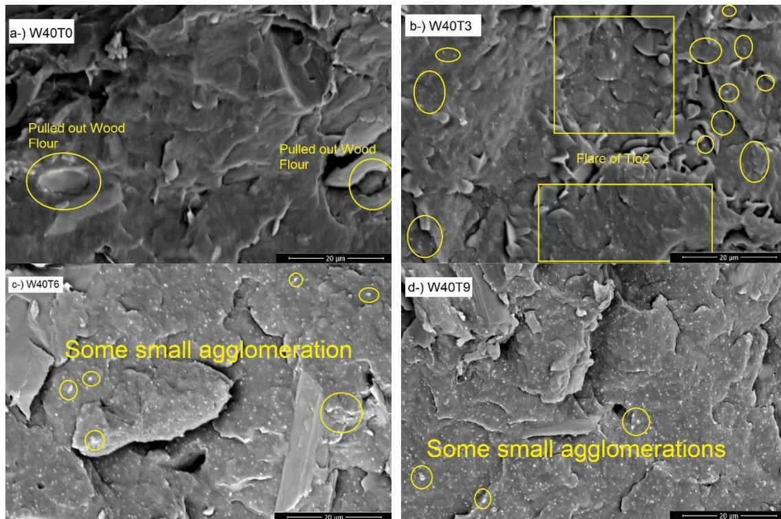
**Fig. 2.** SEM Images (taken at 5000 magnification) of WPCs containing 40% Iroko Flour and different amounts of  $\text{TiO}_2$  taken with a CBS detector: a-) W40T0, b-) W40T3, c-) W40T6, and d-) W40T9
