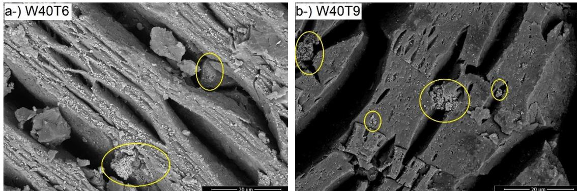
**Fig. 19.** SEM Images (taken at 5000 magnification) of WPCs with a CBS Detector; a-) W40T6, b-) W40T9
