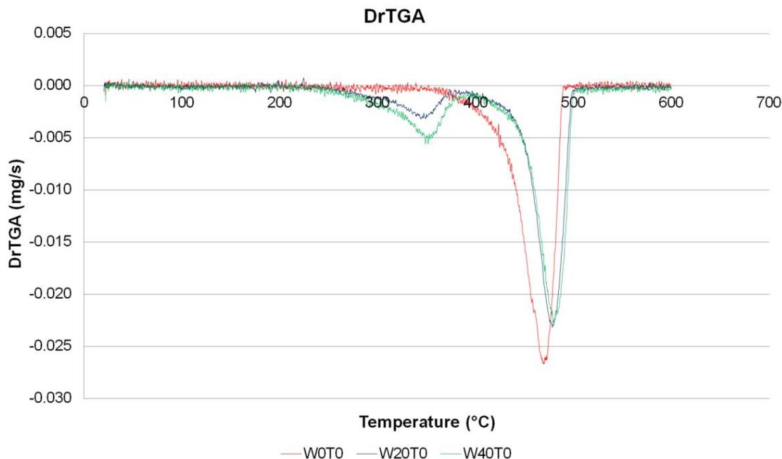
**Fig. 4.** DrTGA results of just WF reinforced PP-based composites
