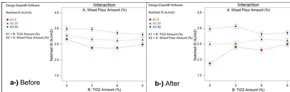
**Fig. 13.** The effects of fillers amount on notched impact strength of WPCs; a-) Before weathering, b-) After weathering
