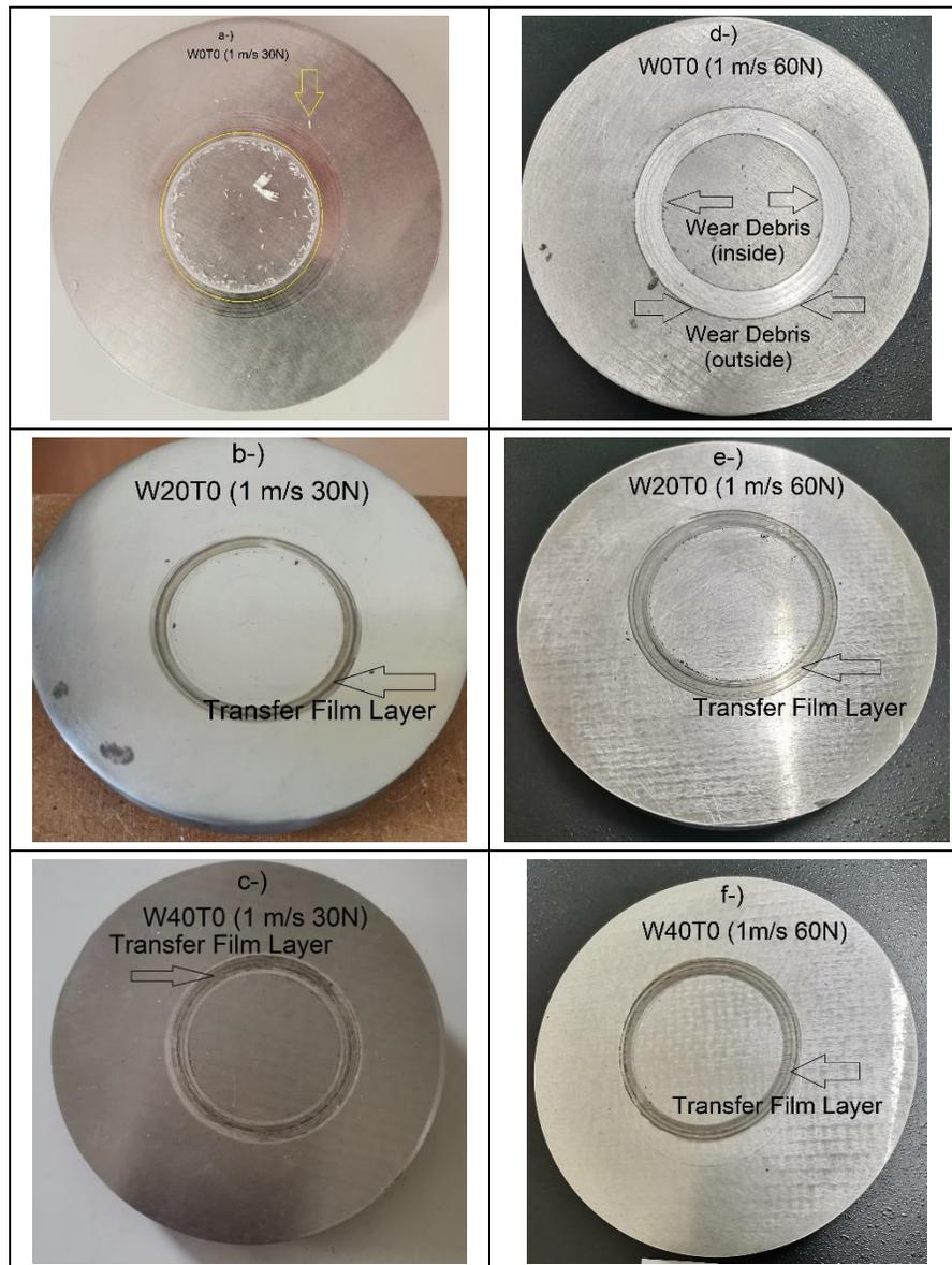
**Fig. 7.** Macro pictures of disc surface of neat PP and wood flour-filled groups: a-) W0T0 (30 N), b-) W20T0 (30 N), c-) W40T0 (30 N), d-) W0T0 (60 N), e-) W20T0 (60 N), and f-) W40T0 (60 N)
