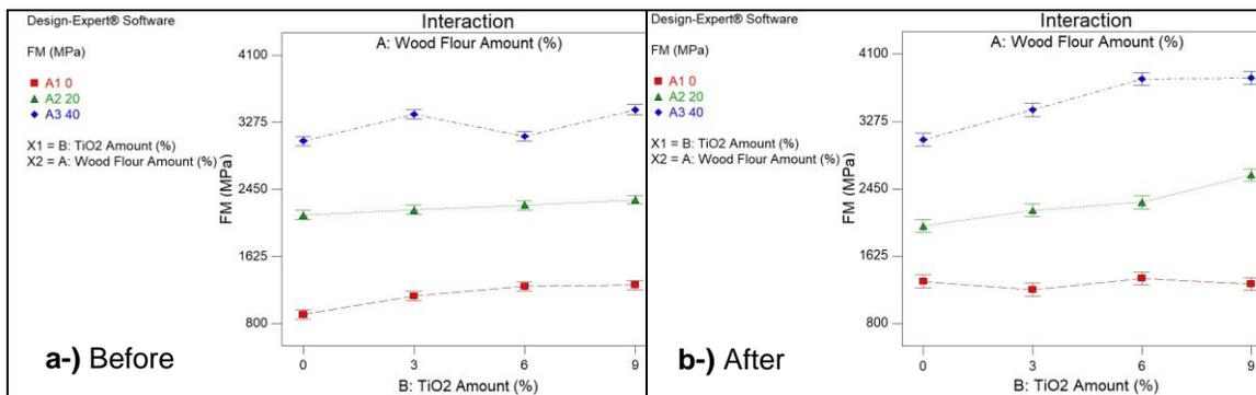
**Fig. 12.** The effects of fillers amount on flexural modulus (MOE) of WPCs; a-) Before weathering, b-) After weathering
