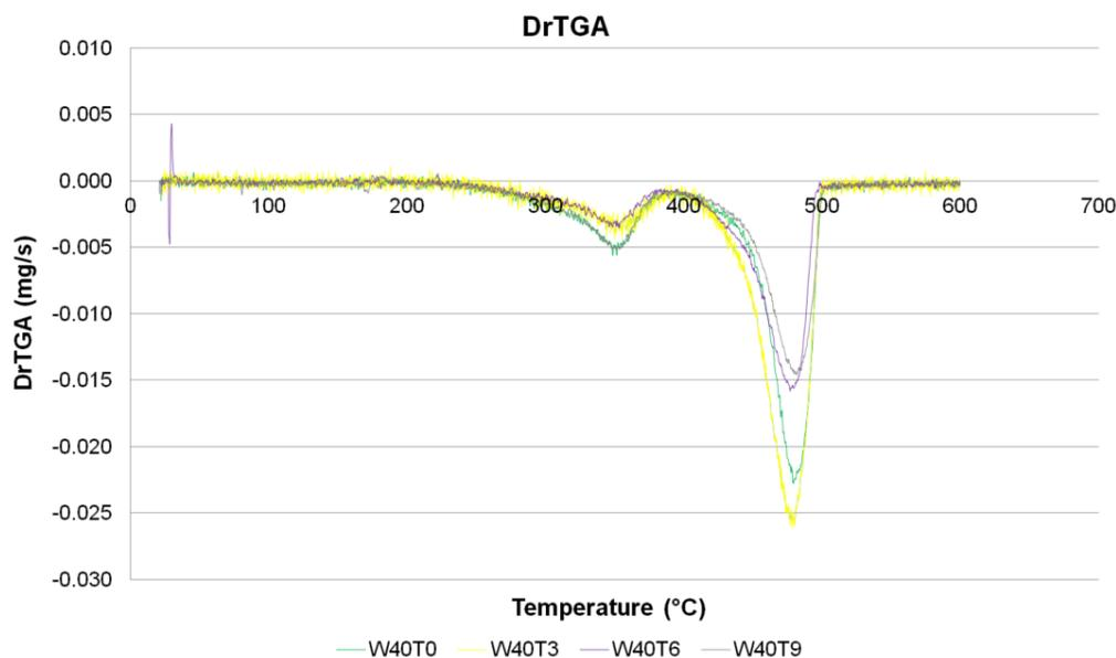
Fig. 5. DrTGA results of PP-based composites contain 40% WF and different amounts of TiO<sub>2</sub>
