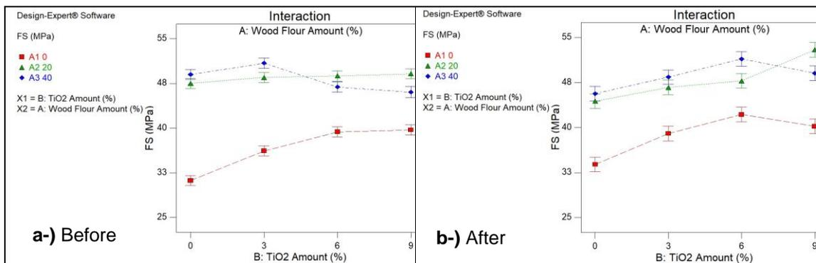
**Fig. 11.** The effects of fillers amount on flexural strength of WPCs: a-) Before weathering, b-) After weathering
