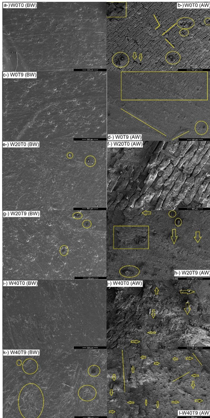
**Fig. 18.** SEM Images (taken at 200 magnification) of WPCs taken before (BW) and after (AW) weathering with a ETD Detector; a-) W0T0 (BW), b-) W0T0 (AW), c-) W0T9 (BW), d-) W0T9 (AW), e-) W20T0 (BW), f-) W20T0 (AW), g-) W20T9 (BW), h-) W20T9 (AW), i-) W40T0 (BW), j-) W40T0 (AW), k-) W40T9 (BW), and l-) W40T9 (AW)
