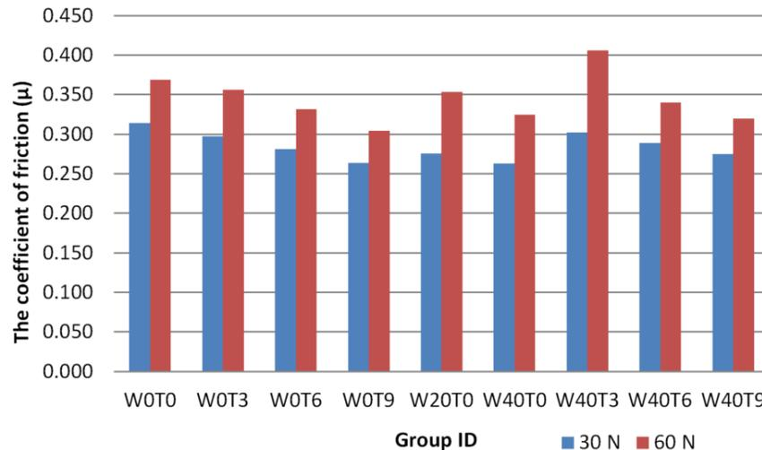
**Fig. 6.** The effect of fillers amount on WPCs friction coefficient
