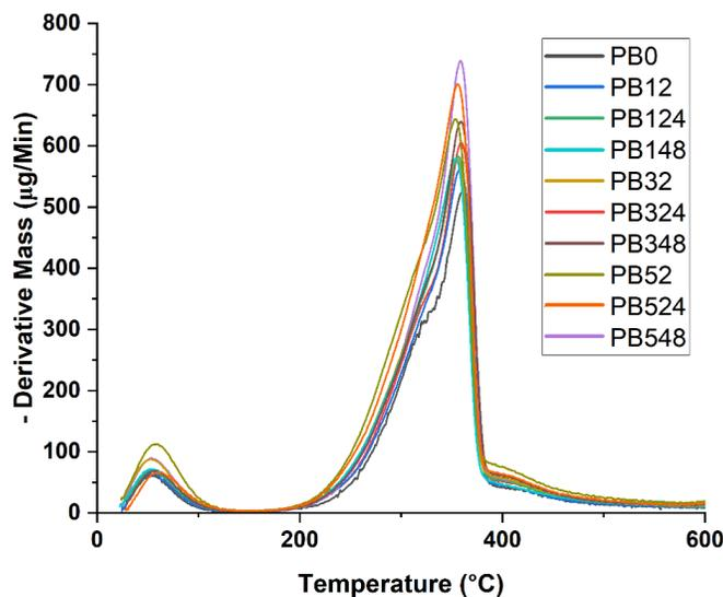
**Fig. 3.** DTG thermograms of the impregnated and non-impregnated brutian pine samples
