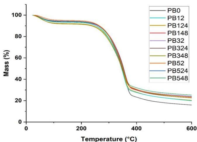
**Fig. 2.** TGA thermograms of the impregnated and non-impregnated brutian pine
