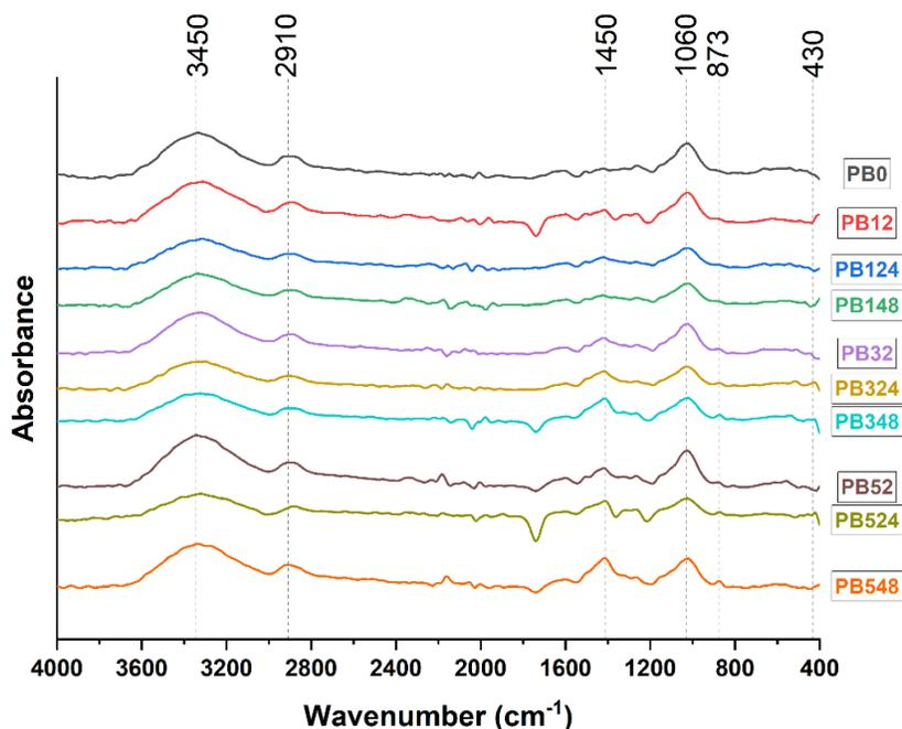
Fig. 1. FTIR spectra of the impregnated and unimpregnated brutian pine samples
