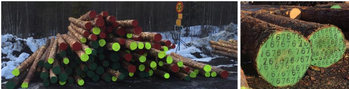
Fig. 1. Half of the logs tested (Scots pine), colored and ID marked to ensure full traceability through the saw line.
