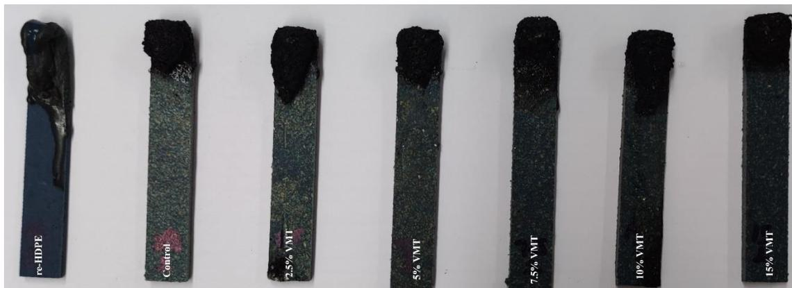
Fig. 4. The LOI samples after testing
